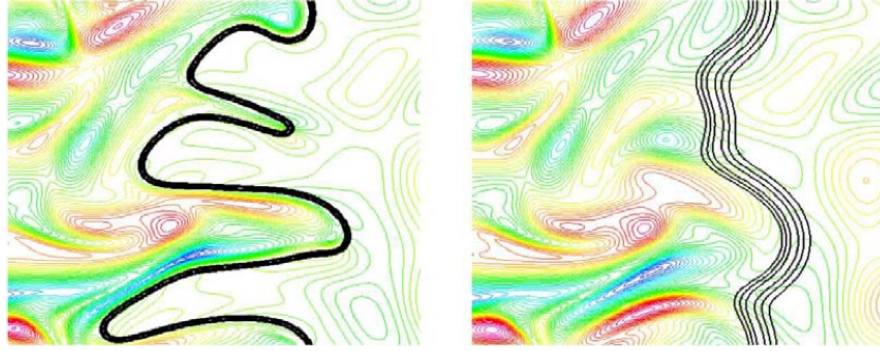
Figure A.1: Reference flame (left) and flame thickened by a factor F = 5 (right). Reaction rate contours are represented in black along with the velocity field from blue to red. From Poinsot & Veynante (2005) .
