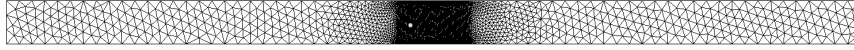
Figure 5.9: Mesh used for the 2D computation. Marker: reference point for n - \tau -model at x = 0.47 .
