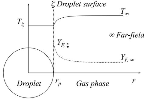
**Figure 3.2:** *Qualitative profiles of temperature  $T$  and fuel mass fraction  $Y_F$  vs radial distance from a spherical single droplet with constant temperature  $T_\zeta$ .*
