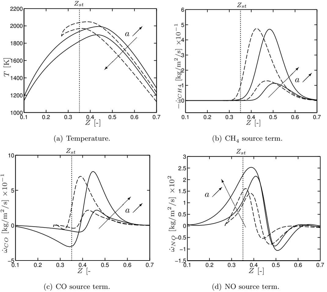
**Figure 8.14: Laminar counterflow flames with ARC\_22\_GRI211.** a) Temperature, b)  $\text{CH}_4$  source term, c) CO source term and d) NO source term vs mixture fraction. Comparison of coflow (—) and pilot (---) counterflow flames at strain rates  $a = 60 \text{ s}^{-1}$  and  $270 \text{ s}^{-1}$ .
