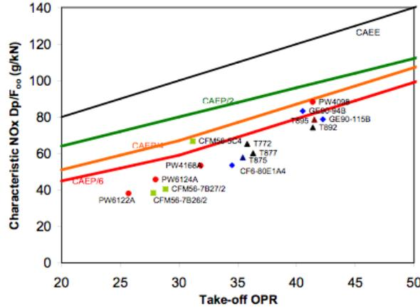
Figure 1.2: NO<sub>x</sub> vs OPR for various engines and comparison with regulatory levels from CAEP. From [1].
