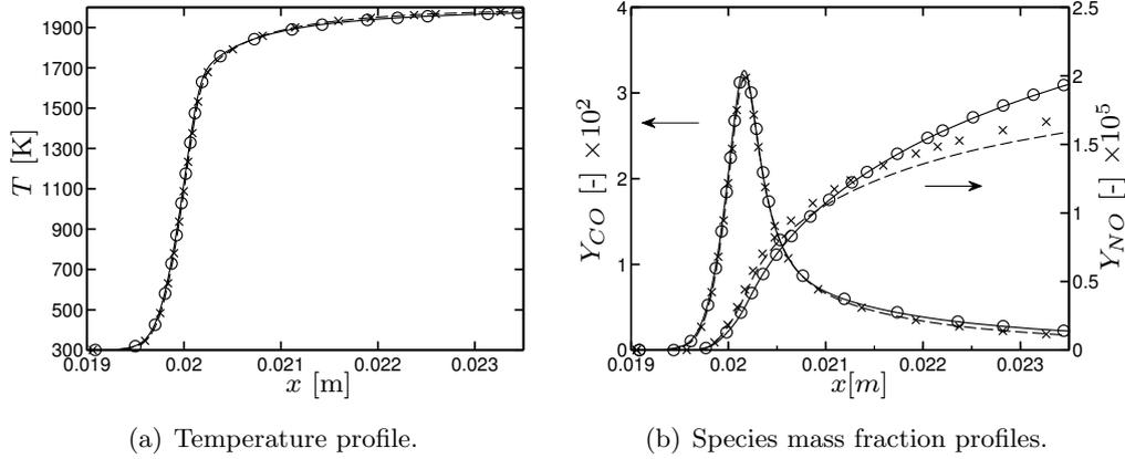
**Figure 6.1:** One-dimensional premixed unstrained methane-air laminar flame in atmospheric conditions at an equivalence ratio  $\phi = 0.8$ . Comparison between GRI 2.11 (—), ARC\_22\_GRI211 ( $\circ$ ), GRI 3.0 (---), ARC\_22\_GRI30 ( $\times$ ).
