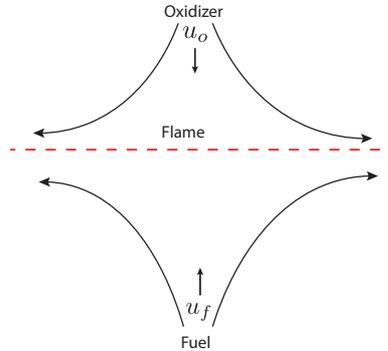
Figure 4.7: Steady strained one-dimensional diffusion flame.
