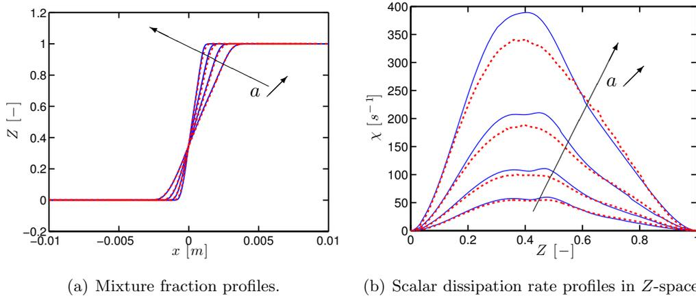
**Figure 7.16:** Counterflow computations in Sandia flame D conditions at global strain rates  $a = 40, 80, 160,$  and  $320 \text{ s}^{-1}$ . Comparison of mixture fraction and scalar dissipation rate profiles from **Cantera** (—) and **AVBP** (···).
