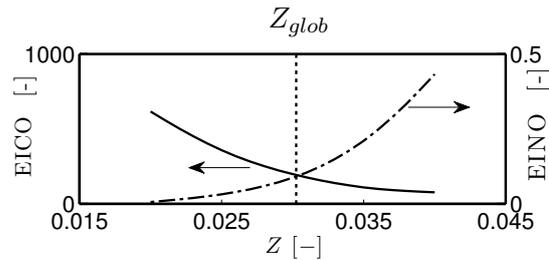
**Figure 9.14: SGT-100/Case A:  $\text{CO}$  ( $\rule{0.5cm}{0.4pt}$ ) and  $\text{NO}$  ( $\rule{0.5cm}{1.2pt}$ ) flame emission indices of unstrained premixed laminar flames vs mixture fraction. The vertical line corresponds to the global mixture fraction.**
