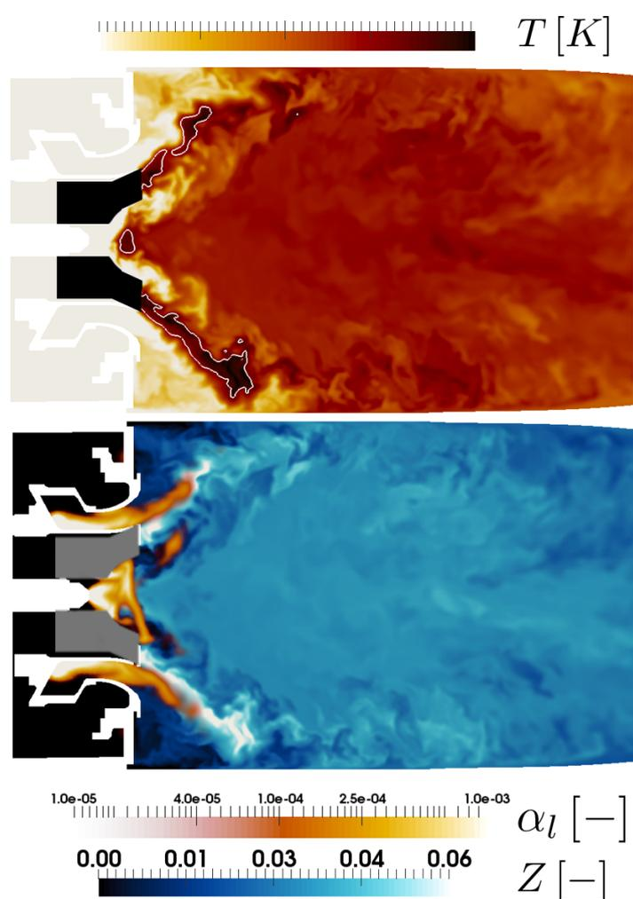
**Figure 10.15:** LEMCOTEC: Top) instantaneous temperature field with  $\phi = 0.8$  isocontour. Bottom) instantaneous field of mixture fraction (blue scale) and superimposed instantaneous field of liquid volume fraction (red scale).
