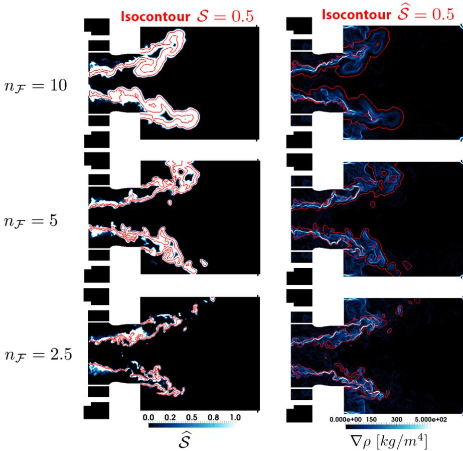
**Figure 9.44: SGT-100/Case A: Instantaneous fields from LES in the mid-plane of the combustor, focused on the first half of the combustor. Left: Filtered thickening sensor  $\hat{\mathcal{S}}$ . Right: density gradient. Comparison between  $n_{\mathcal{F}} = 2.5$  (bottom),  $n_{\mathcal{F}} = 5$  (middle, baseline case) and  $n_{\mathcal{F}} = 10$  (top).**
