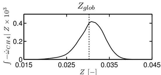
**Figure 9.12: SGT-100/Case A: integrated fuel consumption ( $\text{kg}/\text{m}^3/\text{s}$ ) (—) conditioned on the mixture fraction vs mixture fraction. The vertical line corresponds to the global mixture fraction.**
