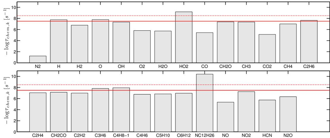
**Figure 10.6:** Species chemical times extracted from a one-dimensional premixed flame at  $\phi = 1.0$  in LEMCOTEC conditions. The continuous line corresponds to the time-step employed in the LES computations ( $\Delta t = 3.0 \times 10^{-8}$  s) and the dotted line to the time-step with 10 chemical subiterations ( $\Delta t^* = \Delta t/10$ ).
