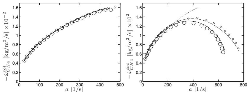
(b) Fuel consumption: coflow (left) and pilot (right) flamelet series.
