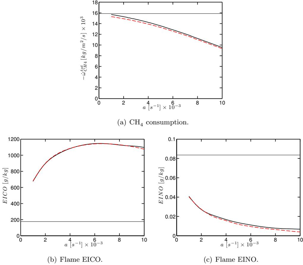
**Figure 9.15: One-dimensional strained premixed flames in SGT-100/Case A conditions at  $\phi = \phi_{glob}$ . Comparison of the response to strain of global quantities between GRI 2.11 (—), ARC\_22\_GRI211 (---). The horizontal lines correspond to the unstrained values for GRI 2.11.**
