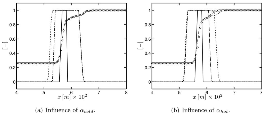
**Figure 6.9: One-dimensional unstrained premixed laminar flame in SGT-100 Case A conditions at  $\phi = 1.0$ . Unfiltered thickening sensor (—), normalised spatial profiles of temperature with baseline parameters (---) and modified parameters ( $\circ$ ), filtered thickening sensor with baseline parameters ( $\cdot\cdot\cdot$ ) and modified parameters ( $-\cdot-$ ).**
