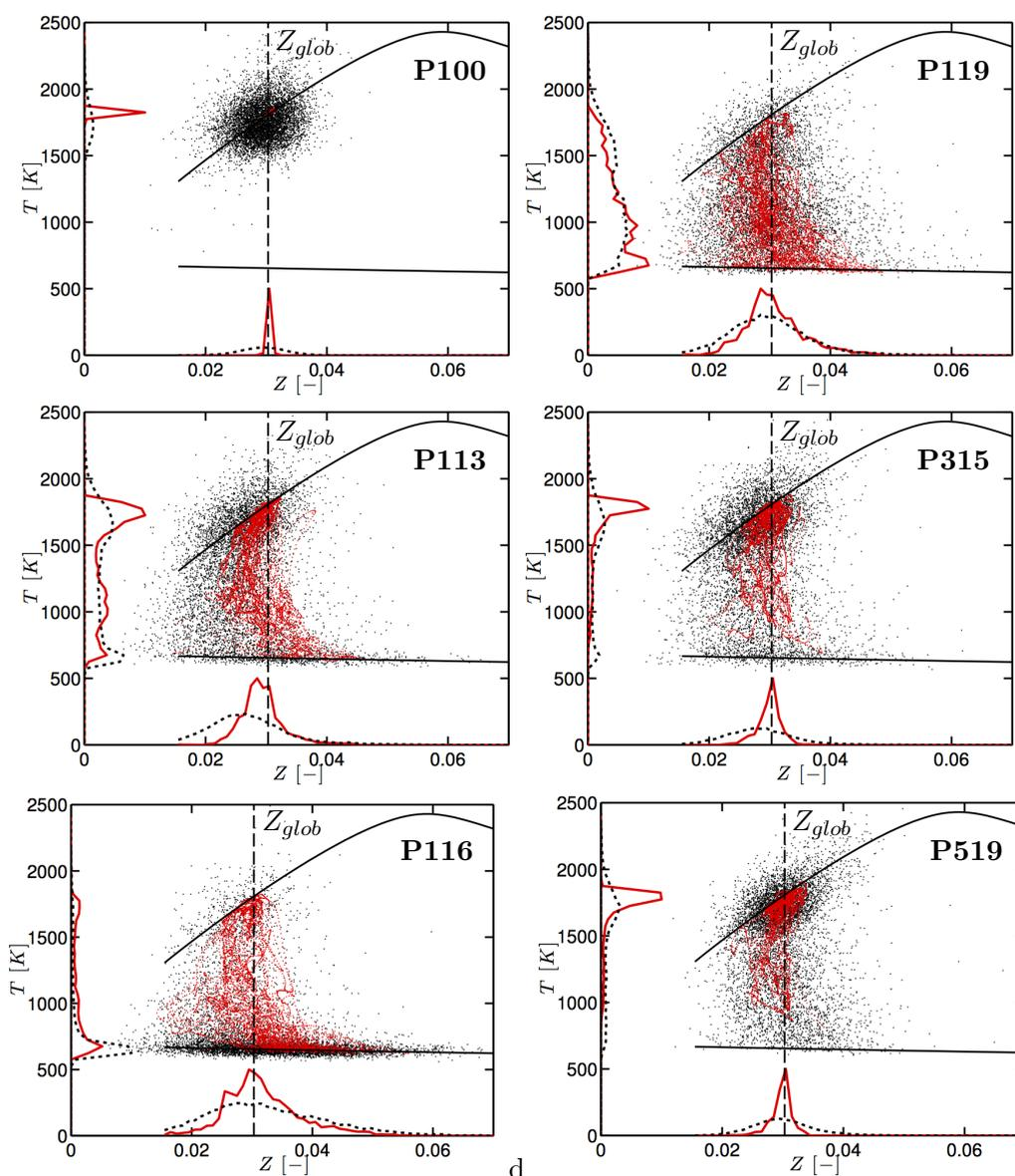
Figure 9.11: SGT-100/Case A: scatter plots of temperature vs mixture fraction at the 6 probes: experiments ( $\cdot$ ) and LES ( $\cdot$ ). PDFs of temperature and mixture fraction are also shown for experiments ( $\cdots$ ) and LES ( $\text{—}$ ). The continuous lines corresponds to equilibrium and mixing lines.
