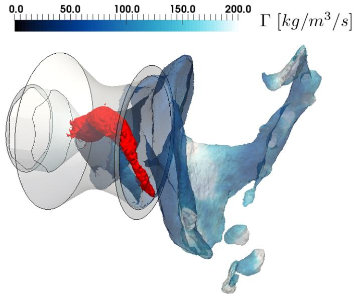
**Figure 10.13:** LEMCOTEC - Pilot injector region: isosurface of stoichiometric liquid volume fraction coloured by evaporation source term and pressure isosurface (red) highlighting the presence of the PVC.
