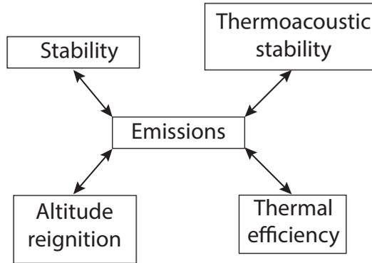
Figure 1.4: Design constraints applying to aeronautical burners.
