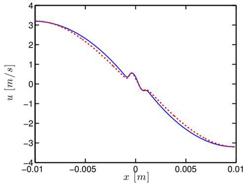
**Figure 7.17:** Counterflow computations in Sandia flame D conditions at global strain rate  $a = 320 \text{ s}^{-1}$ . Comparison of axial velocity profile from **Cantera** (—) and **AVBP** (···).
