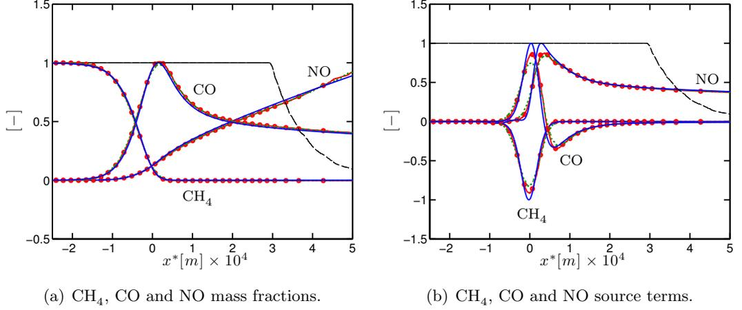
**Figure 7.10:** Three-dimensional premixed plane flame in SGT-100/Case A conditions at  $\phi = 1.0$ . Comparison of mass fraction profiles from **Cantera** (—), **AVBP with source terms @ cells** (—•—) and **AVBP with source terms @ nodes** (···). The thickening sensor  $\theta_F$  (---) profile is also shown. Quantities are normalised by their maximum value obtained with Cantera.
