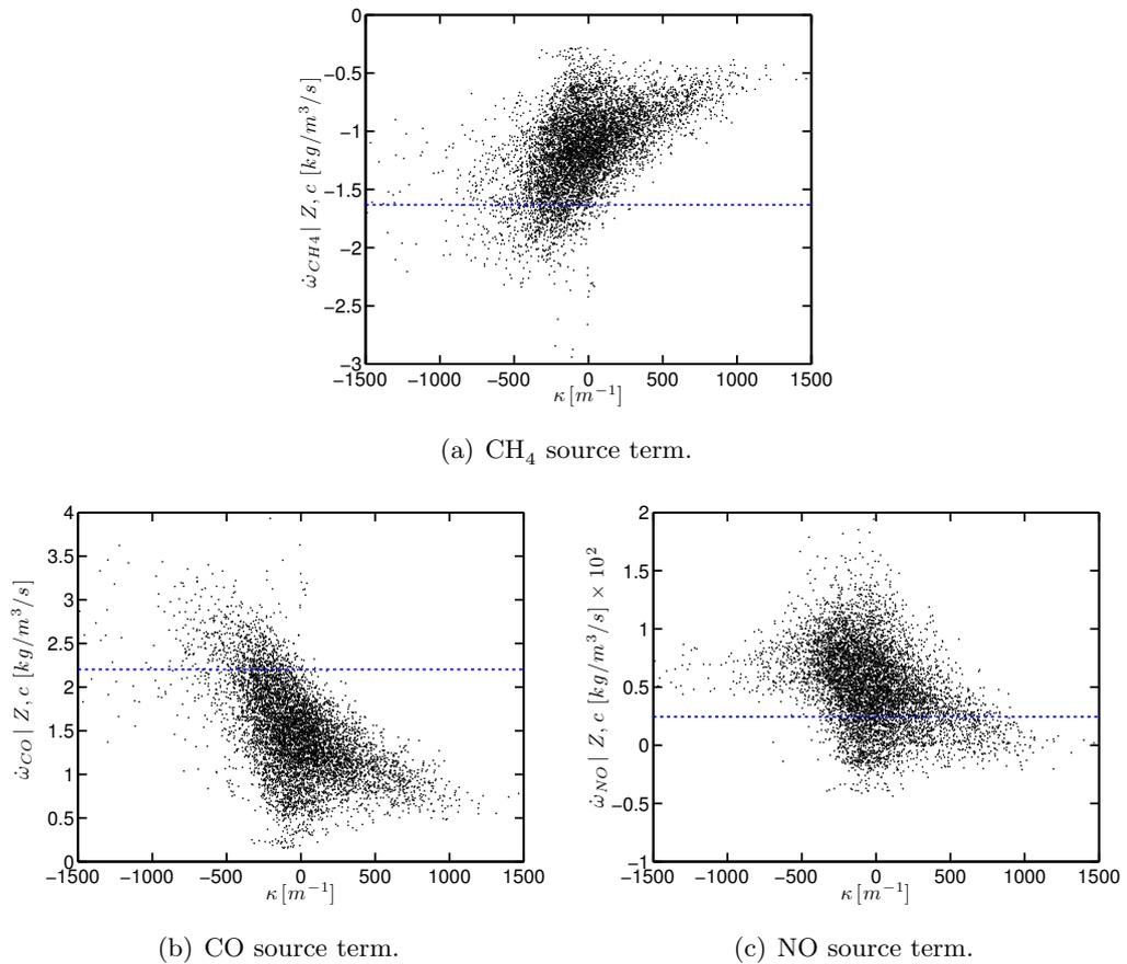
Figure 9.23: SGT-100/Case A: scatter plot ( $\cdot$ ) of a)  $\text{CH}_4$ , b) CO and c) NO instantaneous source terms at  $Z = Z_{glob}$  and  $c = 0.8$  vs curvature. The unstrained laminar premixed flame response ( $\cdot\cdot\cdot$ ) is also shown.
