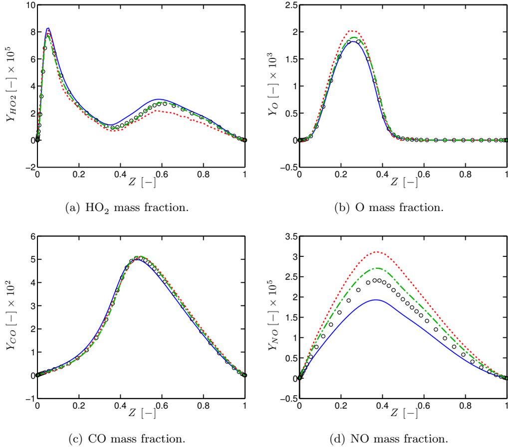
**Figure 7.22:** Counterflow computations in Sandia flame D conditions at global strain rate  $a = 320 \text{ s}^{-1}$ . Comparison of species mass fractions from **Cantera** (—), **AVBP with baseline grid resolution** ( $\Delta x = 0.15 \text{ mm}$ ) (···) in  $Z$ -space and **AVBP with refined grid** ( $\Delta x = 0.075 \text{ mm}$ ) (·-·-·). Cantera flame at global strain rate  $a = 280 \text{ s}^{-1}$  (o) is also shown.
