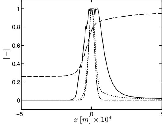
**Figure 6.5: One-dimensional unstrained premixed laminar flame in SGT-100 Case A conditions at  $\phi = 1.0$  with ARC 22.GRI211. Sensor envelope  $\mathcal{T}$  (—),  $\text{CH}_4$  source term (-.-.-), heat release rate (···) and temperature (---) normalised profiles.**
