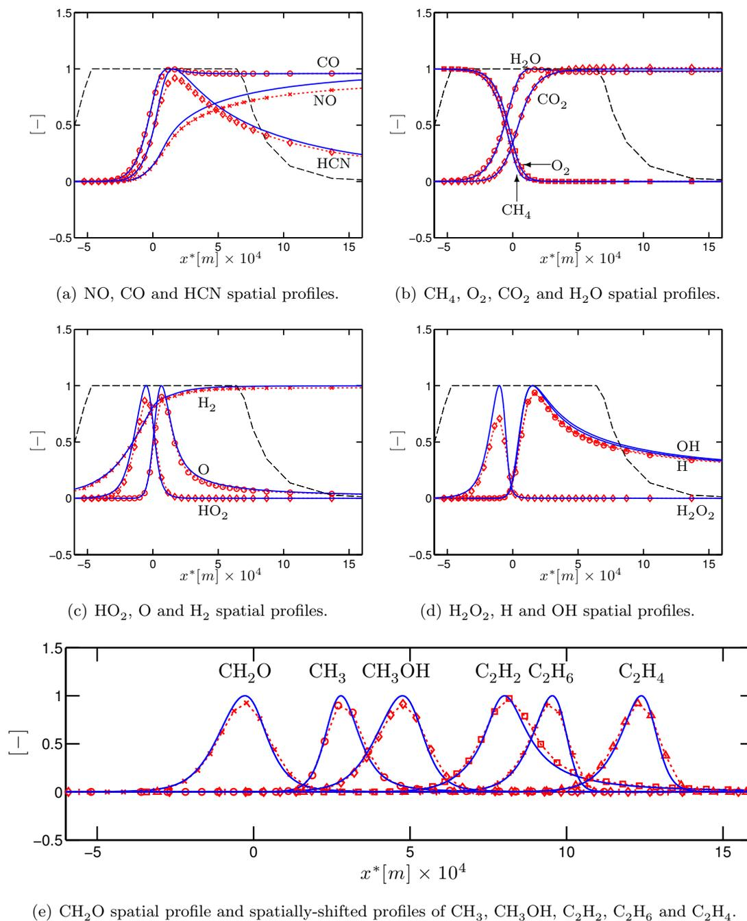
**Figure 7.5:** One-dimensional premixed flame in SGT-100/Case A conditions at  $\phi = 1.4$ . Comparison of mass fraction profiles from **Cantera** (—) and **AVBP** (dotted line with symbols). The thickening sensor  $\theta_F$  (---) profile is also shown. The markers correspond to the grid nodes of the AVBP computation. All the species mass fractions are normalised by their maximum value obtained in Cantera.
