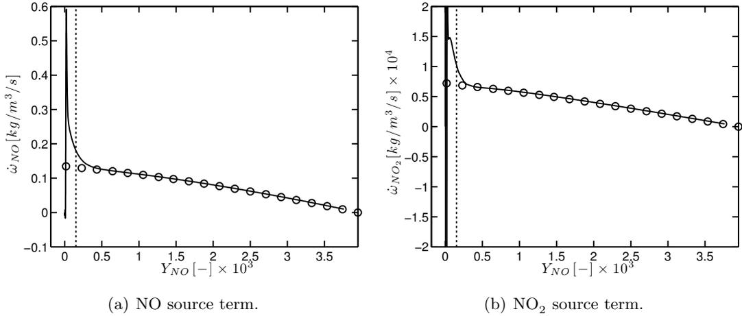
**Figure 5.3:** a) NO source term and b)  $\text{NO}_2$  source term vs NO mass fraction. Comparison between the NOMANI methodology based on premixed flames (—) and the NORA methodology based on PSRs ( $\circ$ ), for a methane-air mixture at  $\phi = 1.0$  ( $T = 680$  K and  $P = 3$  bars - SGT-100 Case A conditions). The vertical line corresponds to  $c = 0.98$ .
