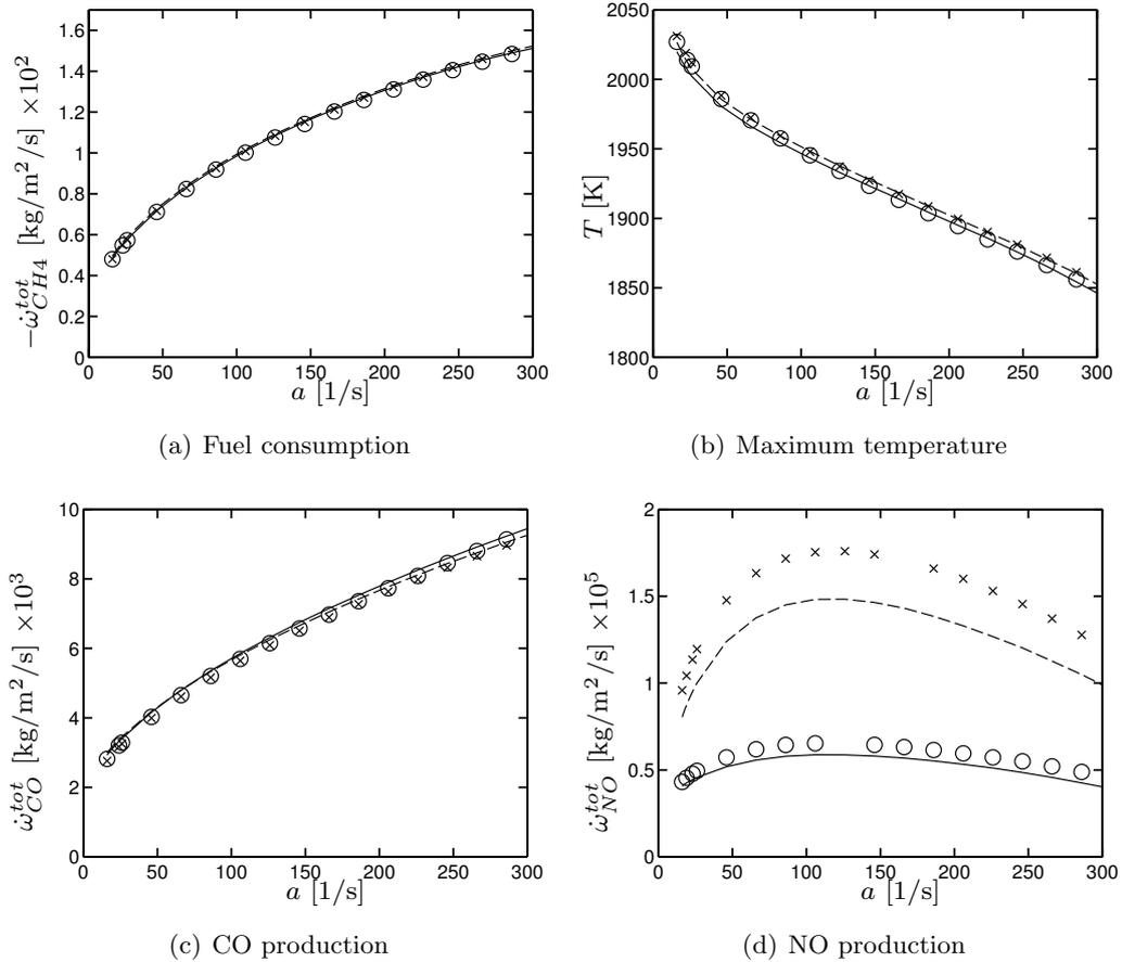
**Figure 7.11: Laminar counterflow diffusion flames in Sandia Flame D conditions. Comparison of the response to global strain rate between GRI 2.11 (—), ARC\_22\_GRI211 (○), GRI 3.0 (---), ARC\_22\_GRI30 (×). in terms of a) total fuel consumption, b) maximum temperature, c) total CO production and d) total NO production.**
