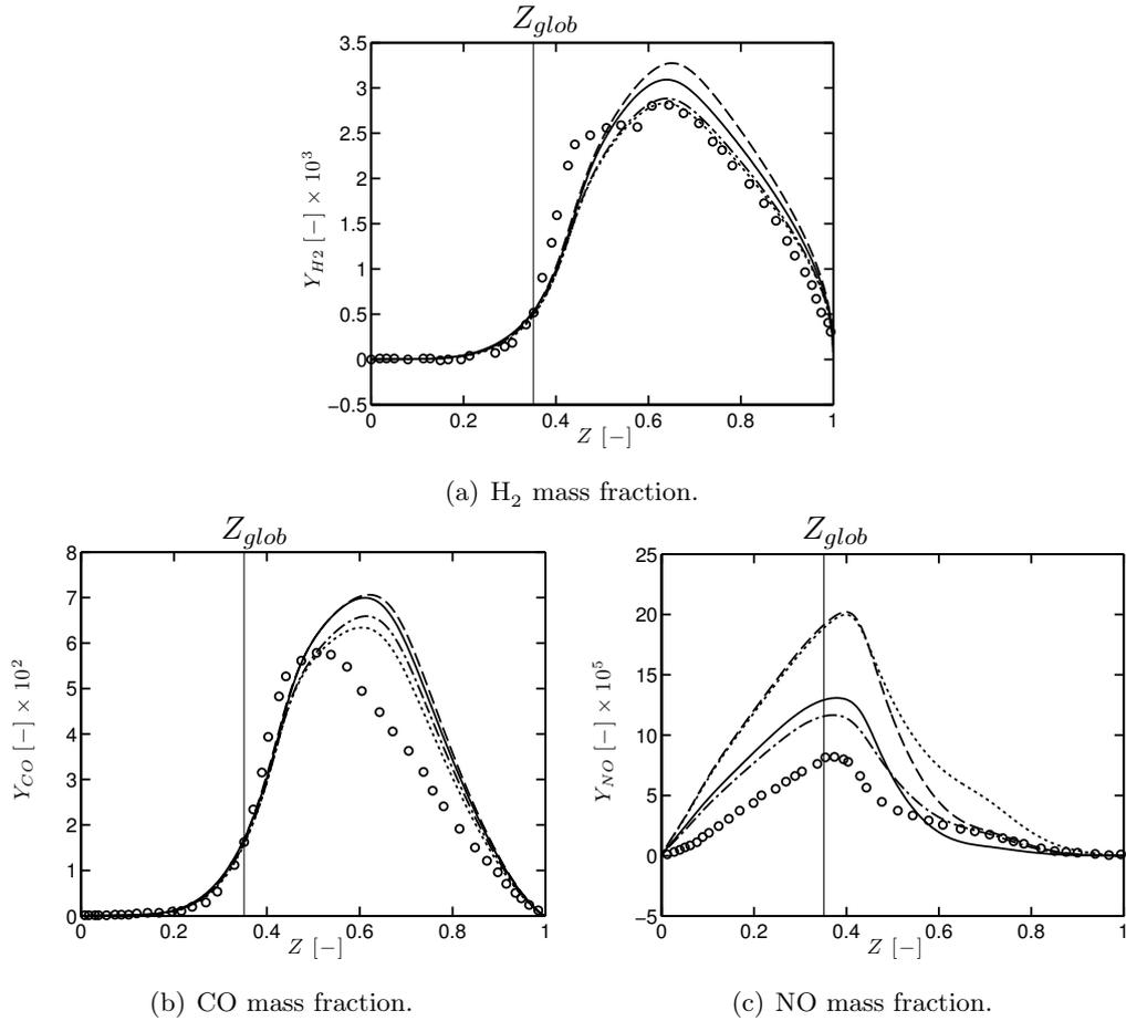
**Figure 7.13: Profiles in  $Z$ -space of a)  $H_2$  mass fraction, b) CO mass fraction and c) NO mass fraction. Comparison between measured profiles from *Barlow et al.* [11] ( $\circ$ ) and computations at global strain rate  $a = 10\text{ s}^{-1}$  with GRI 2.11 (—), ARC\_22\_GRI211 (---), GRI 3.0 (-.-) and ARC\_22\_GRI30 (⋯). The vertical line corresponds to the stoichiometric mixture fraction.**
