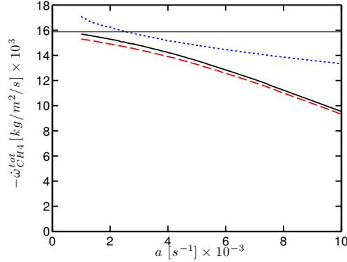
Figure 9.27: One-dimensional strained premixed flames in SGT-100/Case A conditions at  $\phi = \phi_{glob}$ . Comparison of the response to strain of  $\text{CH}_4$  consumption between GRI 2.11 (—), ARC\_22\_GRI211 (---), and 2S\_CH4\_BFER (···). The horizontal line corresponds to the unstrained value for GRI 2.11.
