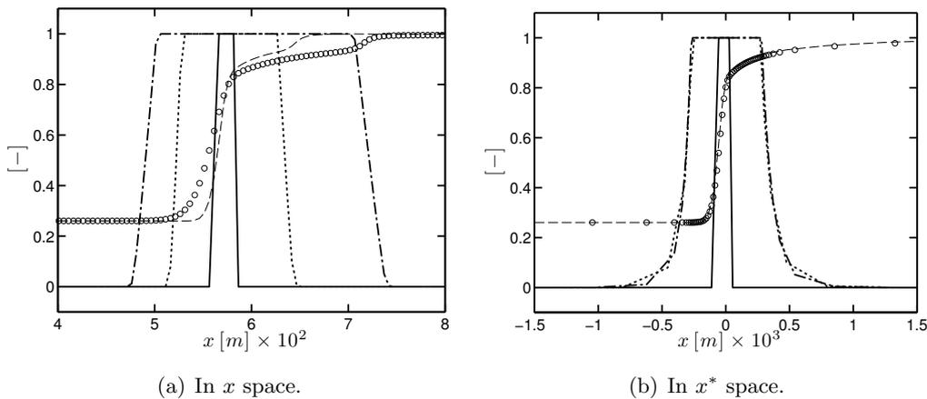
**Figure 6.11:** One-dimensional unstrained premixed laminar flame in SGT-100 Case A conditions at  $\phi = 1.0$ . Unfiltered thickening sensor (—), normalised spatial profiles of temperature with baseline parameters (--) and  $n_{\mathcal{F}} = 10$  ( $\circ$ ), filtered thickening sensor with baseline parameters ( $\cdots$ ) and filtered thickening sensor with  $n_{\mathcal{F}} = 10$  ( $-\cdot-\cdot$ ).
