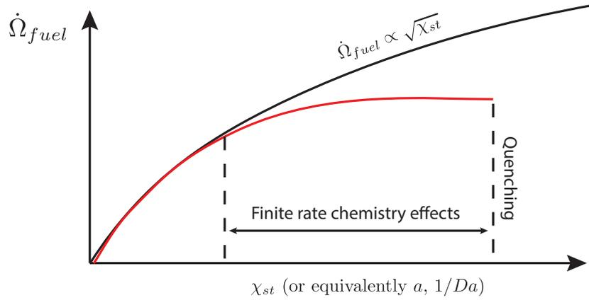
Figure 4.8: Diffusion flame consumption speed vs scalar dissipation (or equivalently strain rate  $a$  or inverse of Damköhler  $1/Da$ ) for infinitely fast chemistry (black) and finite rate chemistry (red).
