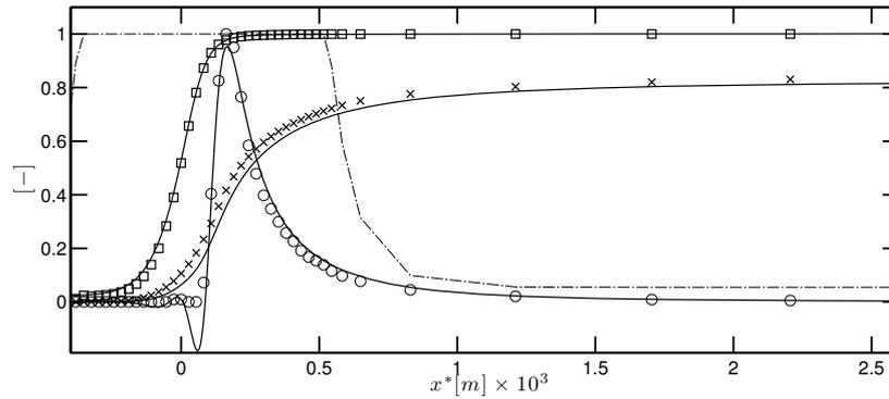
Figure 5.11: Comparison of the NOMAGT model with detailed chemistry on a one-dimensional premixed methane-air flame at  $\phi = 1.4$  with adjusted flame speed: thickening factor (---), progress variable  $c^*$  ( $\square$ ), NO mass fraction from NOMAGT ( $\times$ ) and NO source term from NOMAGT ( $\circ$ ). The continuous lines corresponds to the results obtained for the detailed mechanism with Cantera.
