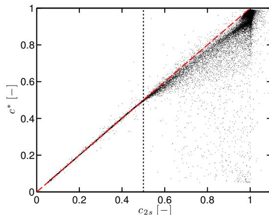
Figure 9.29: SGT-100/Case A - NOMAGT: scatter plot of  $c^*$  vs  $c_{2s}$ . The vertical line corresponds to the switch value  $c_{relax} = 0.5$ . The first bisector ( $c^* = c_{2s}$ ) (—) is also shown.
