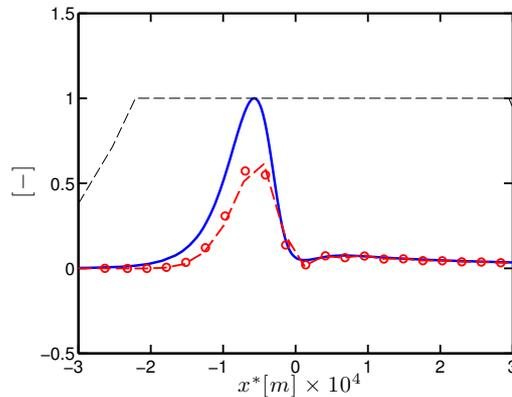
**Figure 7.7:** Effect of temporal integration on one-dimensional premixed flame in SGT-100/Case A conditions at  $\phi = 1.0$ . Comparison of  $\text{H}_2\text{O}_2$  mass fraction profiles from Cantera (—) and AVBP with implicit integration of  $\text{H}_2\text{O}_2$  (--) and explicit integration with  $n_{sub} = 100$  sub-iterations (o). All the species mass fractions are normalised by their maximum value obtained with Cantera.
