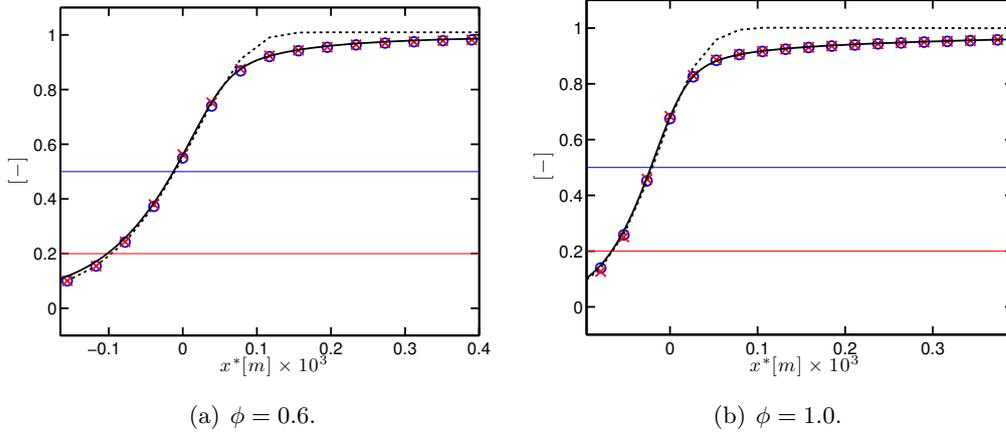
**Figure 5.9:** Comparison of the NOMAGT model with detailed chemistry on a one-dimensional methane-air premixed flame. Impact of  $c_{relax}$  on the progress variable  $c^*$ :  $c_{relax} = 0.5$  ( $\circ$ ), and  $c_{relax} = 0.2$  ( $\times$ ). The progress variable of the reduced chemistry  $c_{2s}$  ( $\cdots$ ) and from the detailed chemistry ( $—$ ) are also shown for comparison. The switch thresholds are indicated by the horizontal lines.
