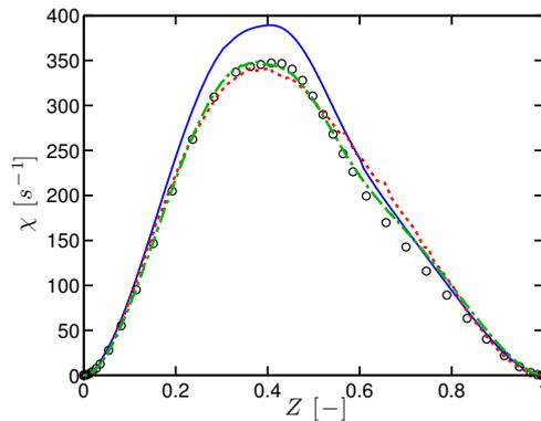
**Figure 7.21:** Counterflow computations in Sandia flame D conditions at global strain rate  $a = 320 \text{ s}^{-1}$ . Comparison of scalar dissipation rate profiles from **Cantera** (—), **AVBP with baseline grid resolution** ( $\Delta x = 0.15 \text{ mm}$ ) ( $\cdot\cdot\cdot$ ) in  $Z$ -space and **AVBP with refined grid** ( $\Delta x = 0.075 \text{ mm}$ ) ( $\cdot - \cdot -$ ). Cantera flame at global strain rate  $a = 280 \text{ s}^{-1}$  ( $\circ$ ) is also shown.
