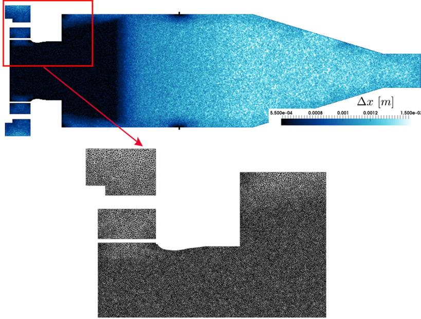
**Figure 9.3: SGT-100: characteristic element size distribution in the mid-plane of the combustor.**
