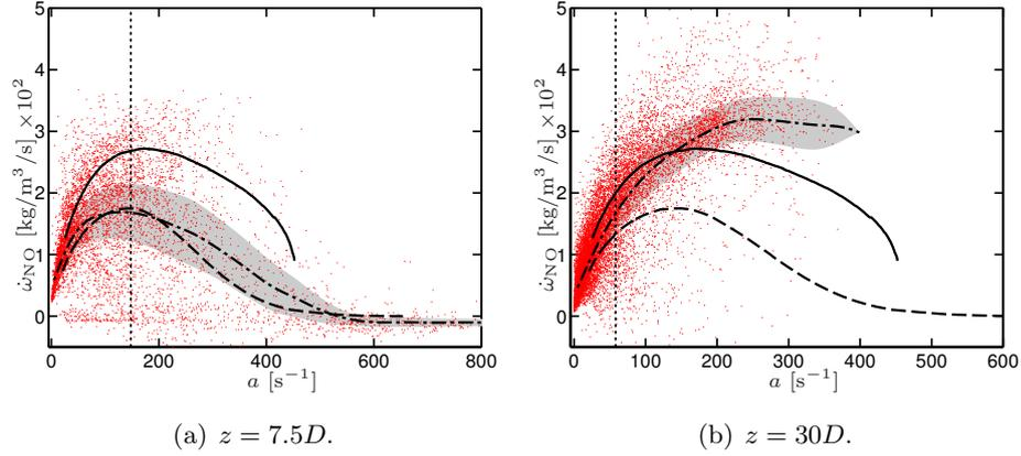
**Figure 8.21: Sandia flame D: Scatter plot of NO production rate versus strain rate along the  $Z = 0.4$  isosurface at axial locations a)  $z = 7.5D$  and b)  $z = 30D$ . The grey shaded area corresponds to the conditional standard deviation around the conditional mean ( $\cdot - \cdot -$ ). The vertical line corresponds to the mean strain rate. LES results are compared to the coflow counterflow flamelets ( $—$ ) and the pilot counterflow flamelets ( $- -$ ).**
