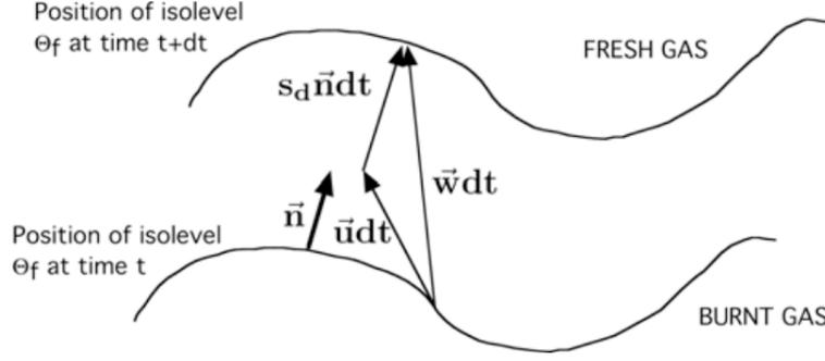
Figure 4.2: Flame speed definitions. From [159].
