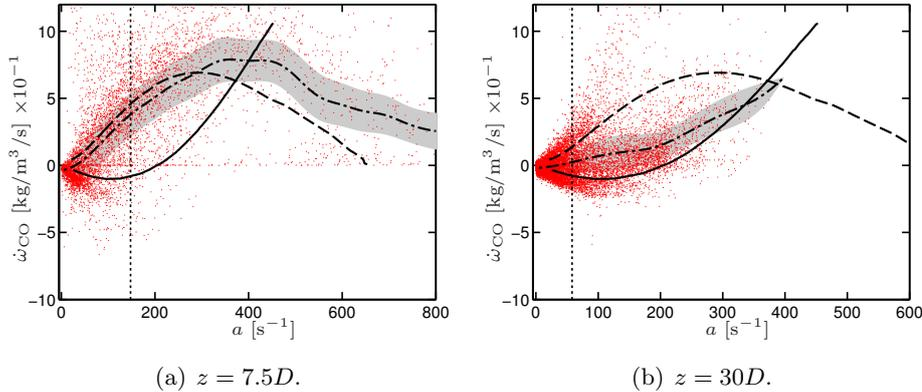
**Figure 8.20: Sandia flame D: Scatter plot of CO production rate versus strain rate along the  $Z = 0.4$  isosurface at axial locations a)  $z = 7.5D$  and b)  $z = 30D$ . The grey shaded area corresponds to the conditional standard deviation around the conditional mean ( $\cdot - \cdot -$ ). The vertical line corresponds to the mean strain rate. LES results are compared to the coflow counterflow flamelets ( $-$ ) and the pilot counterflow flamelets ( $--$ ).**
