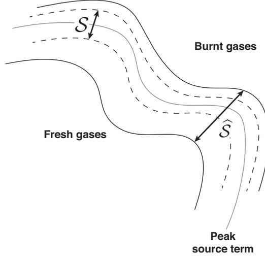
Figure 6.7: Illustration of the sensor filtering procedure.
