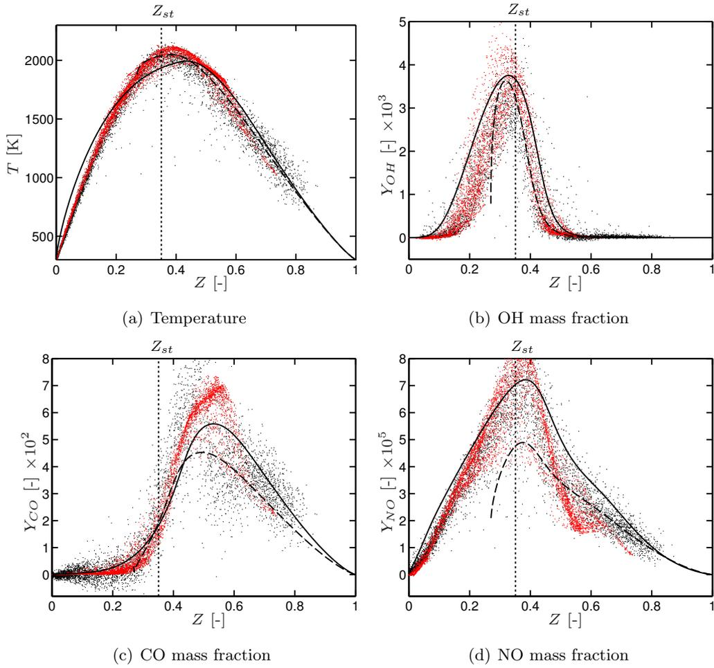
**Figure 8.17: Sandia flame D: Temperature, OH, CO and NO mass fractions vs mixture fraction at axial location  $z = 30D$ . Black dot: experiments, Red dot: LES. Coflow counterflow flame (—) and pilot counterflow flame (---) at strain rate  $a = 60 \text{ s}^{-1}$ .**
