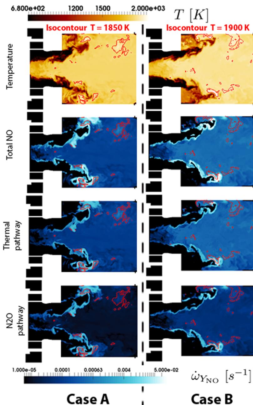
Figure 9.41: SGT-100: Instantaneous fields of temperature, NO source term, thermal and  $N_2O$  pathways. Comparison between Case A and Case B.
