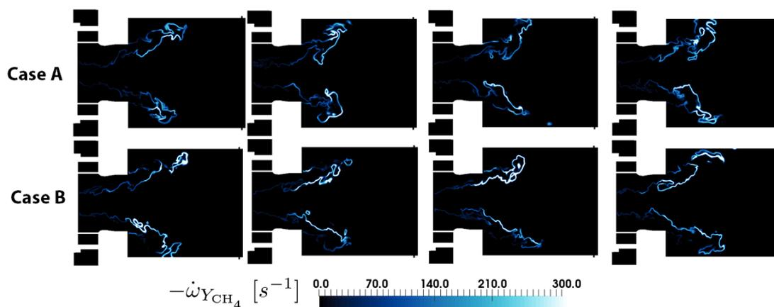
Figure 9.38: SGT-100: Comparison between Case A and Case B: four instantaneous snapshots of  $\text{CH}_4$  destruction rate from LES.
