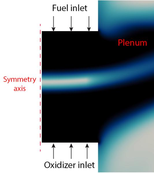
Figure 7.15: Computational domain for two-dimensional counterflow flame.
