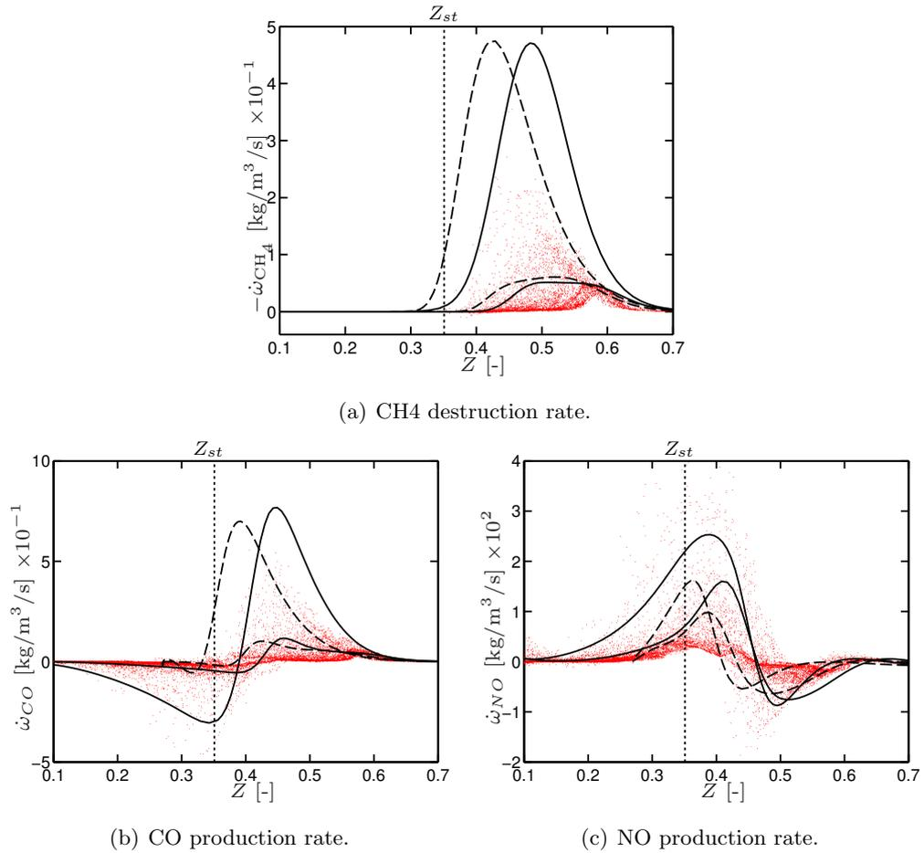
**Figure 8.18: Sandia flame D: Scatter plot of CH<sub>4</sub>, CO and NO source terms vs mixture fraction at axial location  $z = 30D$ . Comparison of coflow (—) and pilot (---) counterflow flames at strain rates  $a = 35 \text{ s}^{-1}$  and  $270 \text{ s}^{-1}$ .**
