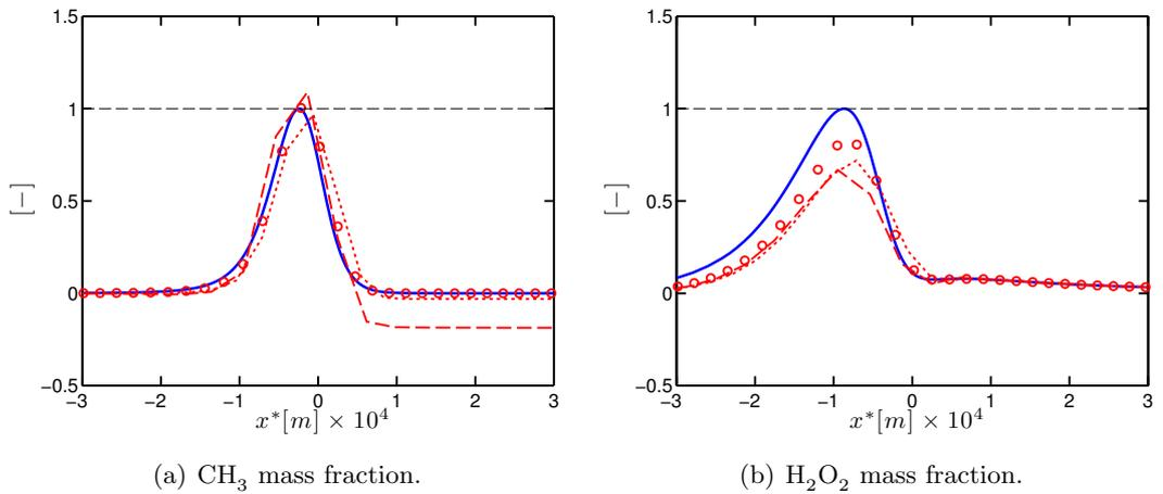
**Figure 7.8:** Effect of grid resolution on one-dimensional premixed flame in SGT-100/Case A conditions at  $\phi = 0.6$ . Comparison of mass fraction profiles from **Cantera** (—) and **AVBP** with  $n_{\mathcal{F}} = 5$  (---),  $n_{\mathcal{F}} = 7.5$  (··) and  $n_{\mathcal{F}} = 10$  (o). The species mass fractions are normalised by their maximum value obtained with Cantera.
