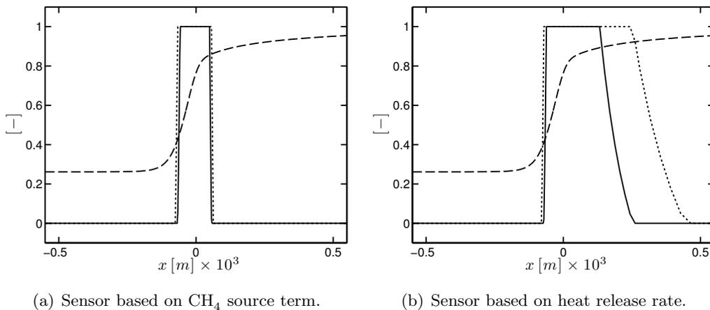
**Figure 6.6:** One-dimensional unstrained premixed methane-air laminar flame in SGT-100 Case A conditions at  $\phi = 1.0$ . Normalised spatial profiles of temperature (---), thickening sensor (—) and thickening sensor with  $\sigma \rightarrow \sigma/2$  (···) based a) on fuel source term and b) on heat release rate.
