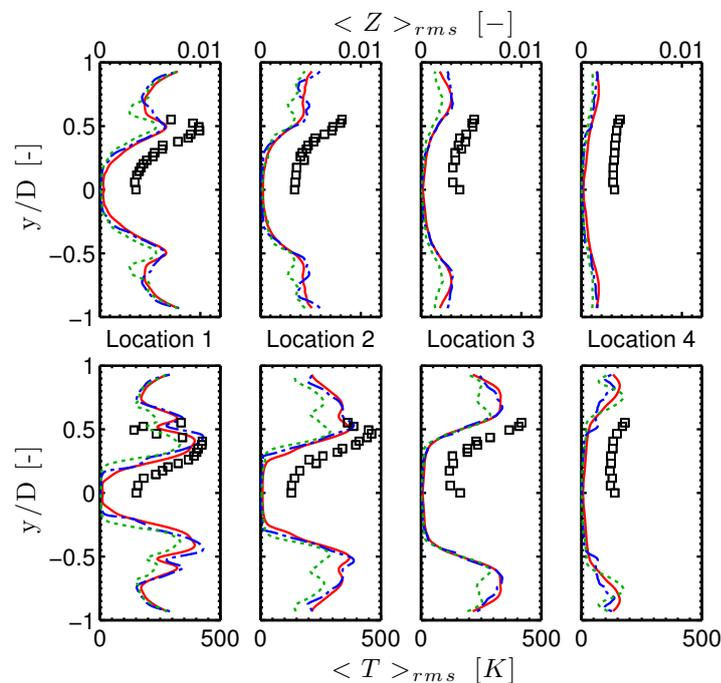
Figure 9.47: SGT-100/Case A: Transverse profiles of rms mixture fraction (top) and rms temperature (bottom). Comparison between **LES with  $n_{\mathcal{F}} = 5$**  (—), **LES with  $n_{\mathcal{F}} = 2.5$**  (---), **LES with  $n_{\mathcal{F}} = 10$**  (···) and experiments ( $\square$ ).
