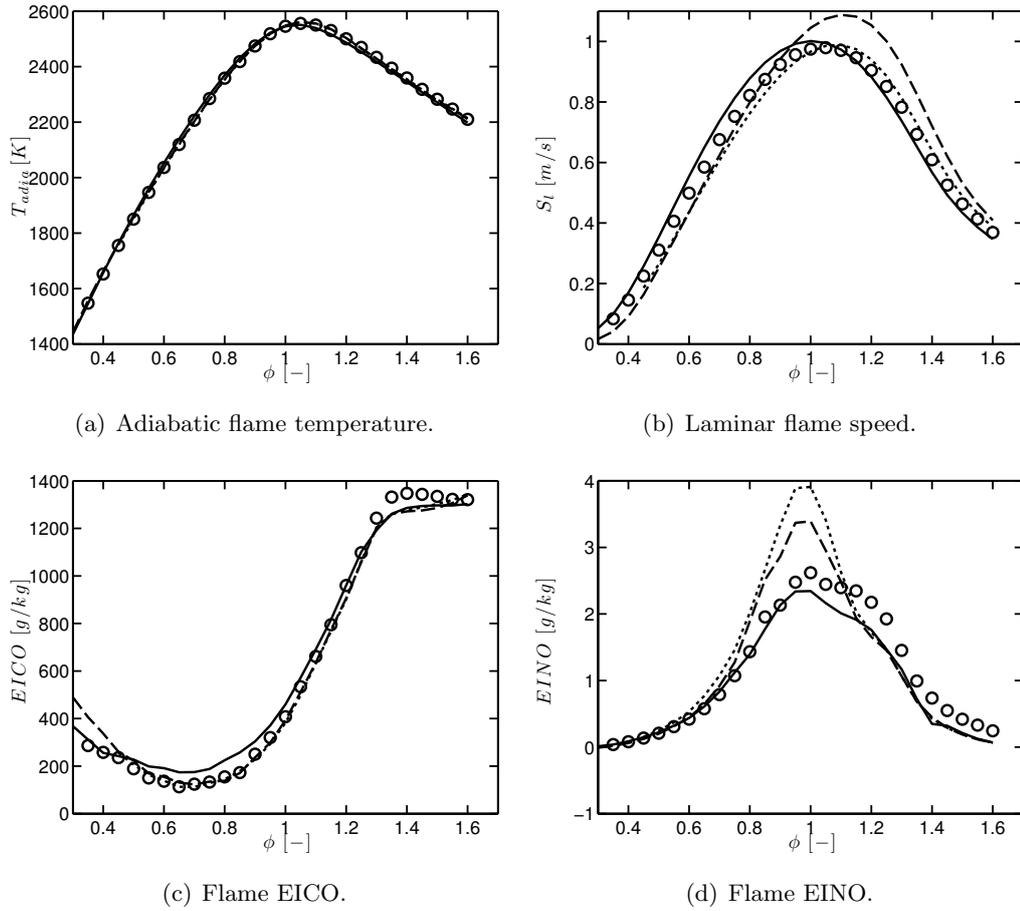
**Figure 10.4: Laminar unstrained premixed flames in LEMCOTEC conditions.** Comparison of a) adiabatic flame temperature, b) laminar flame speed, c) flame EICO and d) flame EINO between JetSurf mechanism (—), Dagaut mechanism ( $\cdots$ ), Luche mechanism (---) and ARC\_27\_JETSURF ( $\circ$ ).
