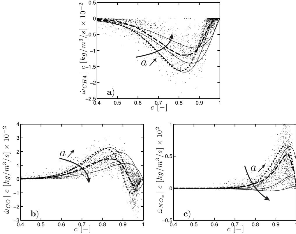
**Figure 9.19: SGT-100/Case A: Scatter plot (·) and conditional mean (—) of a) CH<sub>4</sub>, b) CO and c) NO<sub>x</sub> instantaneous source terms conditionally averaged on progress variable and mixture fraction  $Z_{glob}$ . The unstrained laminar premixed flame response (▪▪) and strained laminar premixed flame cases (—) at strain rate  $a = 1000, 6000, 11000 \text{ s}^{-1}$  are also shown for comparison.**
