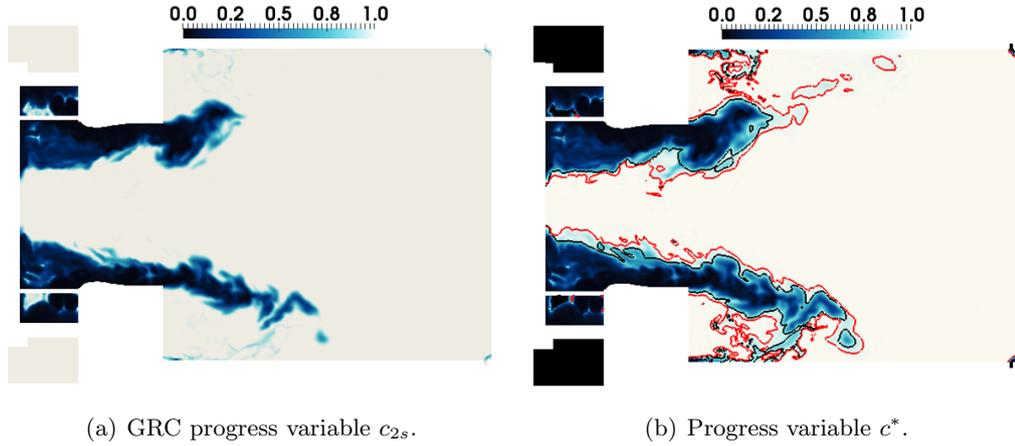
Figure 9.28: SGT-100/Case A - NOMAGT: Instantaneous fields of a) progress variable from 2-step chemistry  $c_{2s}$  and b) progress variable  $c^*$  with  $c_{2s} = 0.98$  isocontour (black) and  $c^* = 0.98$  isocontour (red).
