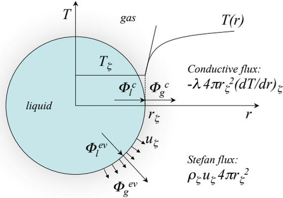
**Figure 3.3:** Contributions to the enthalpy balance at the liquid-gaseous interface
