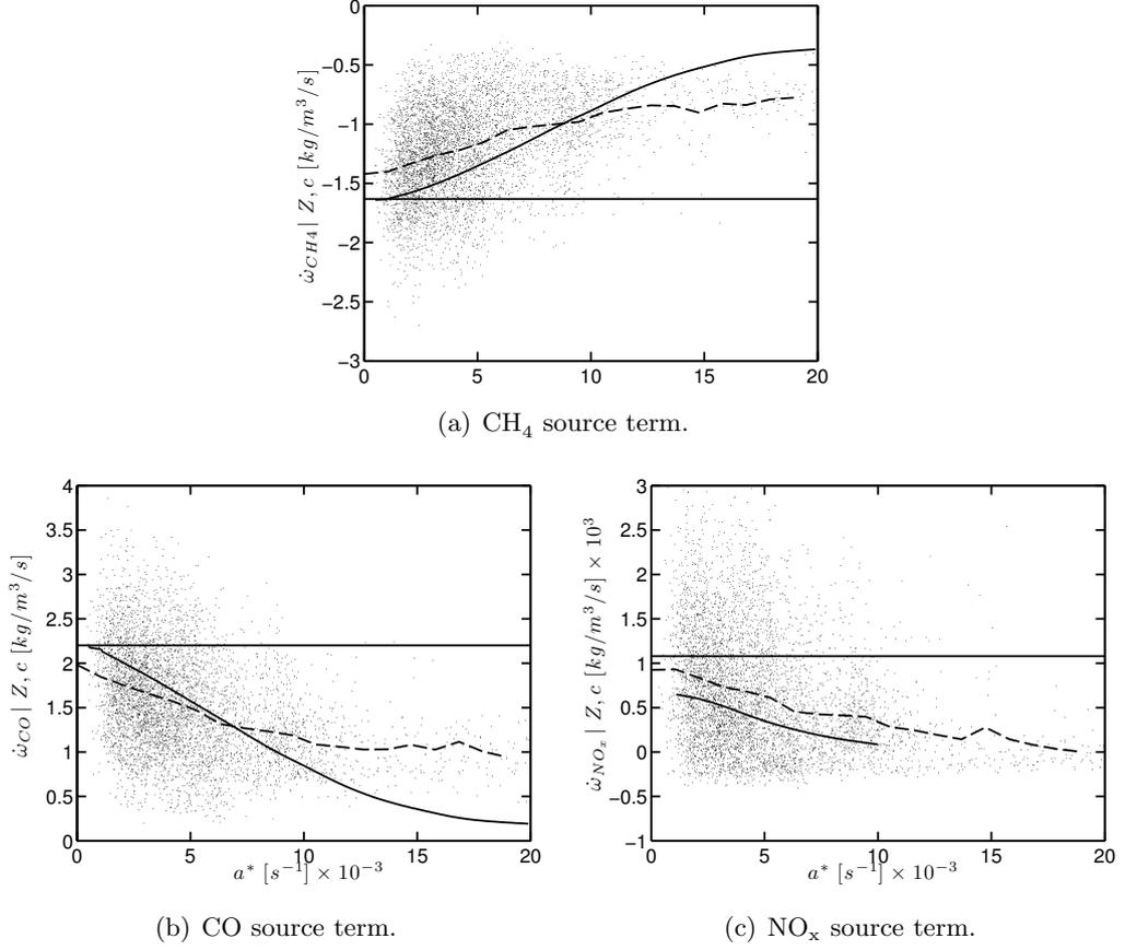
**Figure 9.20: SGT-100/Case A: Scatter plot at mixture fraction value  $Z_{glob}$  and progress variable value  $c = 0.8$  of a) CH<sub>4</sub>, b) CO and c) NO<sub>x</sub> instantaneous source terms vs effective mean-velocity strain rate  $a^*$ . LES data are conditionally averaged (---) on the effective mean-velocity strain rate. The strained laminar premixed flame response (—) and unstrained response (horizontal line) are also shown for comparison.**
