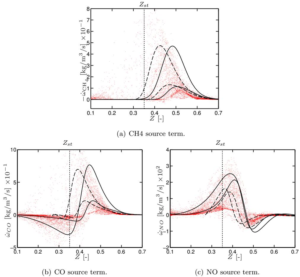
**Figure 8.16: Sandia flame D: Scatter plot of  $\text{CH}_4$ , CO and NO source terms vs mixture fraction at axial location  $z = 7.5D$ . Comparison of coflow (—) and pilot (---) counterflow flames at strain rates  $a = 60\text{ s}^{-1}$  and  $270\text{ s}^{-1}$ .**
