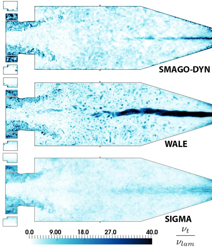
Figure 9.43: SGT-100/Case A: instantaneous fields of turbulent to laminar viscosity ratio  $\mathcal{R}$  in the mid-plane of the combustor. Comparison between Dynamic Smagorinsky (top), WALE (middle) and SIGMA (bottom) subgrid scale models.
