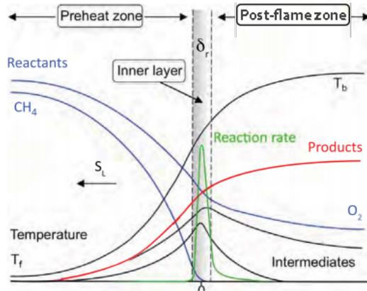
Figure 4.1: Schematic of a one-dimensional premixed  $\text{CH}_4/\text{air}$  flame.
