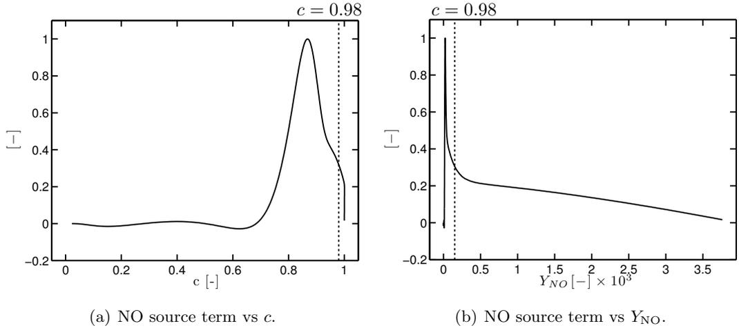
**Figure 5.2: One-dimensional premixed methane-air flame at  $\phi = 1.0$  ( $T = 680$  K and  $P = 3$  bars - SGT-100 conditions). NO source term vs a) progress variable  $c$  and b) NO mass fraction  $Y_{\text{NO}}$ . Quantities are normalised by their extrema. The vertical line corresponds to  $c = 0.98$ .**
