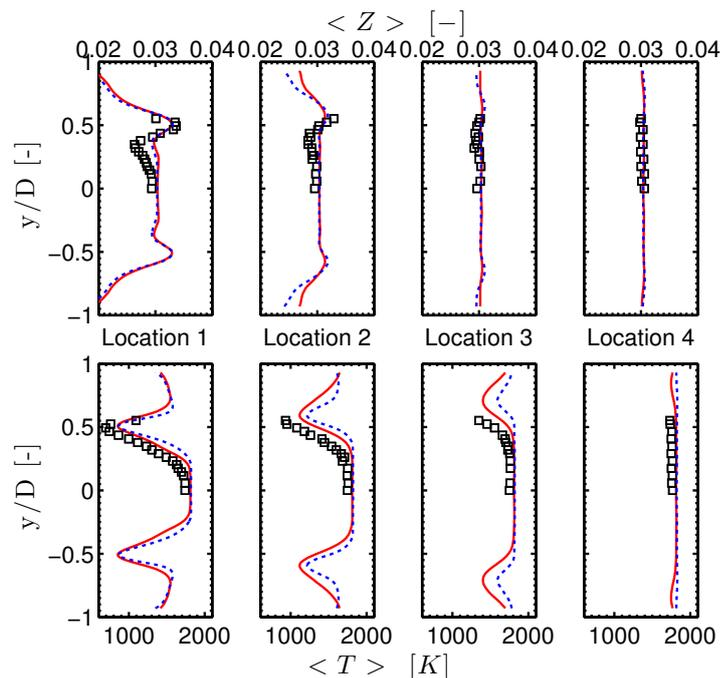
Figure 9.24: SGT-100/Case A - NOMAGT: Transverse profiles of mean mixture fraction (top) and temperature (bottom). Comparison between **LES with ARC** (—), **LES with GRC** (---) and experiments ( $\square$ ).
