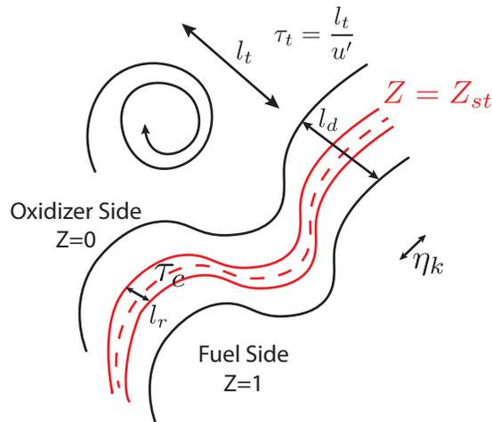
Figure 4.9: Spatial scales in turbulent diffusion flames. Turbulent scales: Integral length scale  $l_t$ , integral time scale  $\tau_t$  and Kolmogorov scale  $\eta_k$ . Flame scales: diffusive thickness  $l_d$ , reaction zone thickness  $l_r$  and chemical time  $\tau_c$ .
