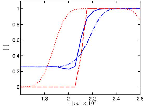
Figure 6.4: One-dimensional unstrained premixed laminar flame in SGT-100 Case A conditions at  $\phi = 1.0$  with 2S\_CH4\_BFER mechanism. Comparison of normalised spatial profiles of temperature (Standard method: —, “Gather/Scatter” method: - - -) and thickening sensor (Standard method: --, “Gather/Scatter” method: ···).
