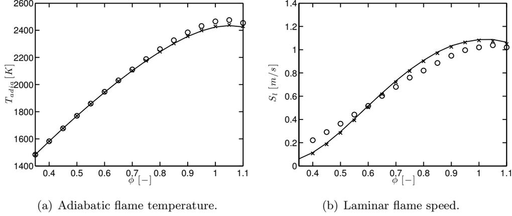
**Figure A.1: One-dimensional unstrained premixed methane-air laminar flames in the SGT-100 Case A conditions. Comparison between GRI 2.11 detailed mechanism (—), ARC 22\_GRI211 (×) and 2S\_CH4\_BFER scheme (○) for a) adiabatic flame temperature and b) laminar flame speed.**
