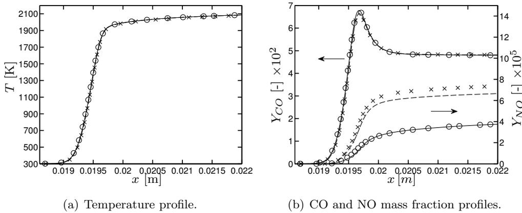
**Figure 6.2:** One-dimensional premixed unstrained methane-air laminar flame in atmospheric conditions at an equivalence ratio  $\phi = 1.2$ . Comparison between GRI 2.11 (—), ARC\_22\_GRI211 ( $\circ$ ), GRI 3.0 (---), ARC\_22\_GRI30 ( $\times$ ).
