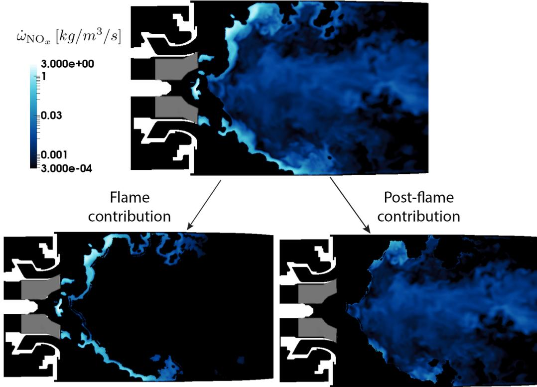
Figure 10.22: LEMCOTEC: Instantaneous NO source term (log-scale) in the mid-plane of the combustor. Decomposition into fast flame and slow post-flame contributions based on the thickening sensor.
