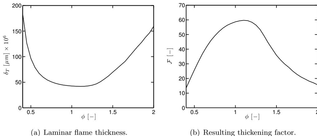
**Figure 10.11: Laminar flame thickness from one-dimensional premixed flame computations in LEMCOTEC conditions and resulting thickening factor vs equivalence ratio ( $\Delta x = 0.5$  mm and  $n_{\mathcal{F}} = 5$ ).**
