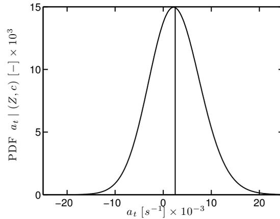
**Figure 9.17: SGT-100/Case A: PDF of instantaneous tangential strain rate  $a_t$  (—) conditioned on  $Z = Z_{glob}$  and  $c = 0.8$ . The vertical line correspond to the spatial mean value  $a_t^{mean} = 2500 \text{ s}^{-1}$ .**
