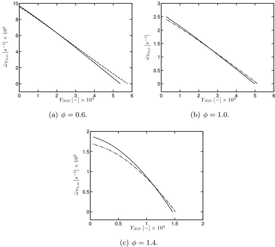
**Figure 10.5: Evolution of NO source term in phase space extracted from PSR calculations after an initial perturbation of equilibrium composition, for three equivalence ratios. Comparison between Luche mechanism (—) and ARC\_27\_JETSURF (· - · -).**
