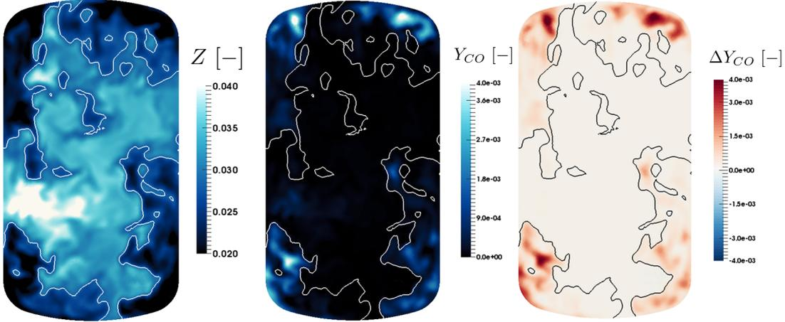
Figure 10.18: LEMCOTEC: Instantaneous LES fields in the exit plane of the combustor. Left: Mixture fraction with isocontour at  $Z = Z_{glob}$ . Middle: CO mass fraction. Right: CO deviation from equilibrium.
