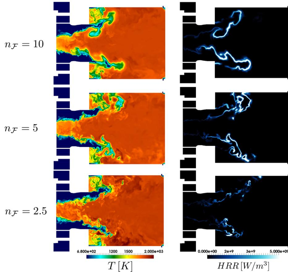
**Figure 9.45: SGT-100/Case A: Instantaneous fields from LES in the mid-plane of the combustor, focused on the first half of the combustor. Left: temperature. Right: heat release rate. Comparison between  $n_{\mathcal{F}} = 2.5$  (bottom),  $n_{\mathcal{F}} = 5$  (middle, baseline case) and  $n_{\mathcal{F}} = 10$  (top).**
