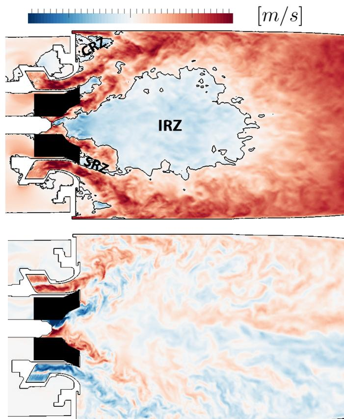
**Figure 10.12: LEMCOTEC: Instantaneous fields of axial velocity with zero axial velocity isocontour (top) and tangential velocity (bottom) from LES. CRZ: Corner Recirculation Zone. IRZ: Inner Recirculation Zone. SRZ: Separator Recirculation Zone.**
