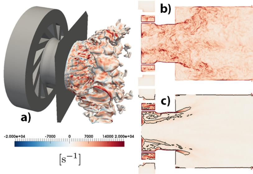
**Figure 9.18: SGT-100/Case A: a) Instantaneous field of tangential strain rate on  $c = 0.8$  isosurface. b) maximum strain rate of instantaneous velocity field and c) maximum strain rate of mean-velocity field in the mid-plane of the combustor.**
