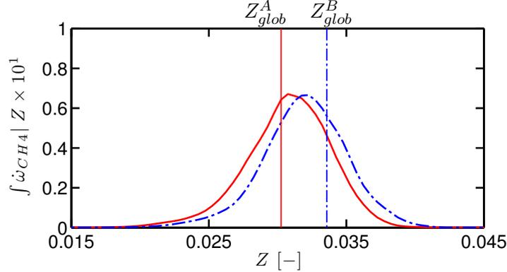
Figure 9.39: SGT-100: Normalised integrated fuel consumption conditioned on the mixture fraction vs mixture fraction. Comparison between **Case A** (—) and **Case B** (· - · -). The vertical lines correspond to the respective global mixture fraction of both cases.
