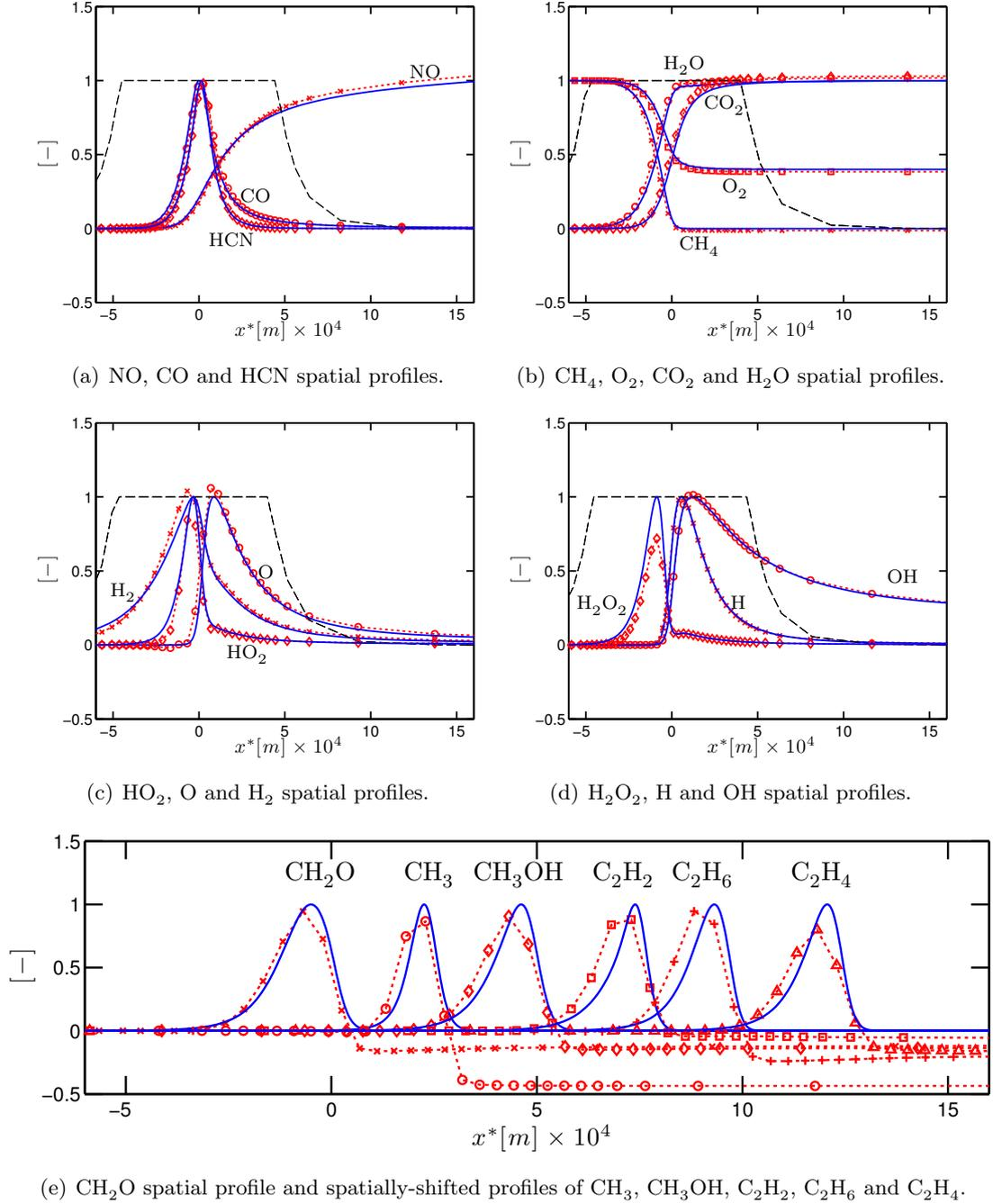
**Figure 7.4:** One-dimensional premixed flame in SGT-100/Case A conditions at  $\phi = 0.6$ . Comparison of mass fraction profiles from **Cantera** (—) and **AVBP** (dotted line with symbols). The thickening sensor  $\theta_F$  (---) profile is also shown. The markers correspond to the grid nodes of the AVBP computation. All the species mass fractions are normalised by their maximum value obtained in Cantera.
