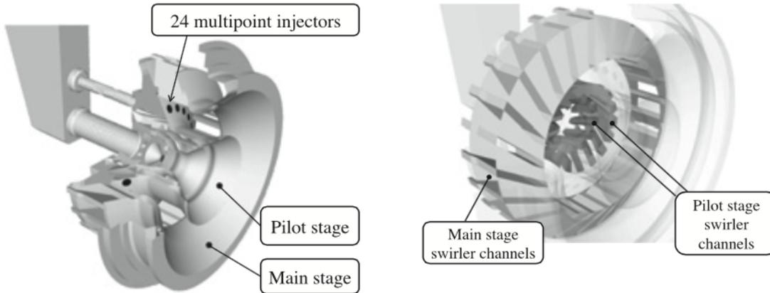
**Figure 1.7: SNECMA multipoint injector design (TLC project). From [91].**
