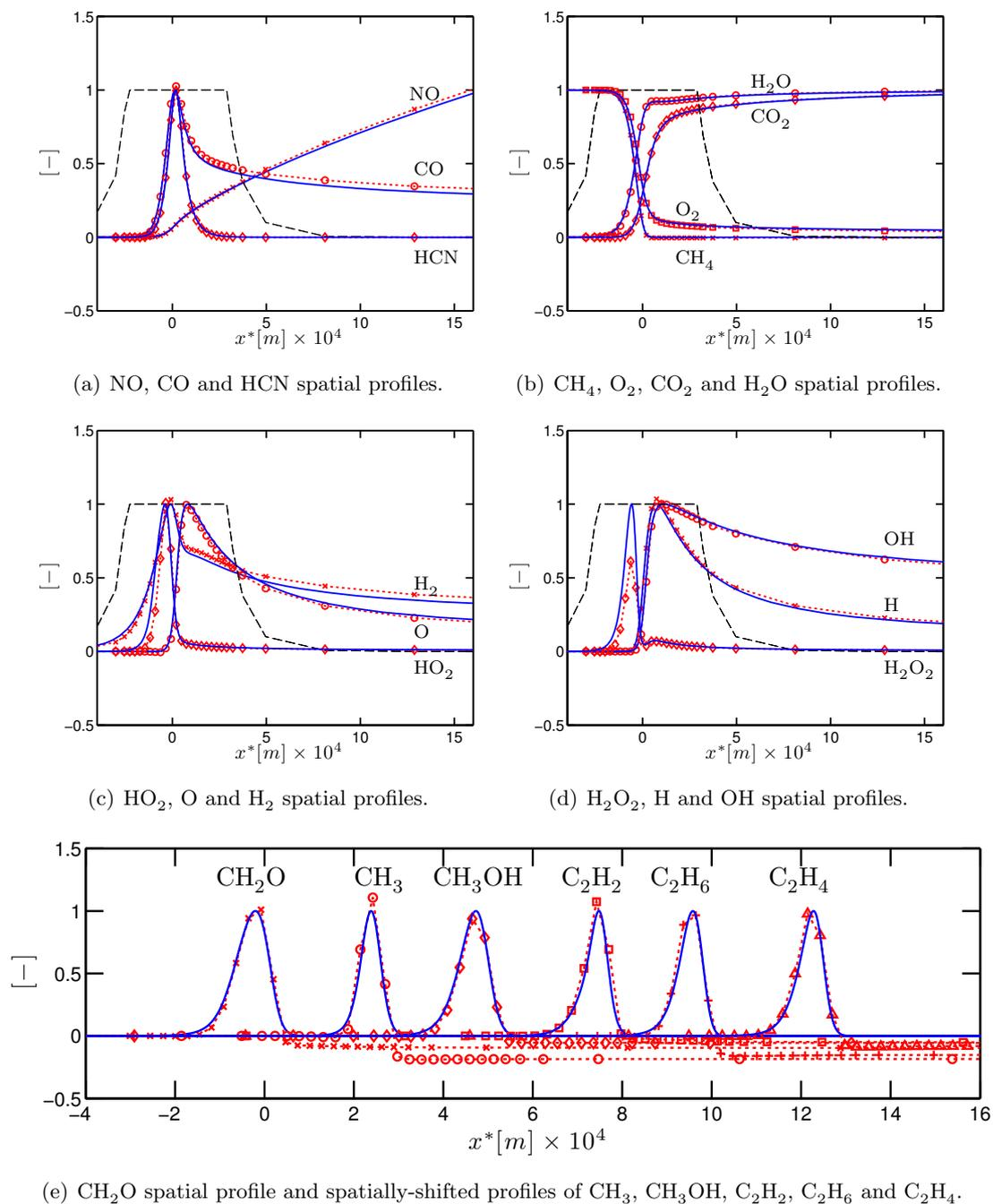
**Figure 7.3:** One-dimensional premixed flame in SGT-100/Case A conditions at  $\phi = 1.0$ . Comparison of mass fraction profiles from **Cantera** (—) and **AVBP** (dotted line with symbols). The thickening sensor  $\theta_F$  (---) profile is also shown. The markers correspond to the grid nodes of the AVBP computation. All the species mass fractions are normalised by their maximum value obtained in Cantera.
