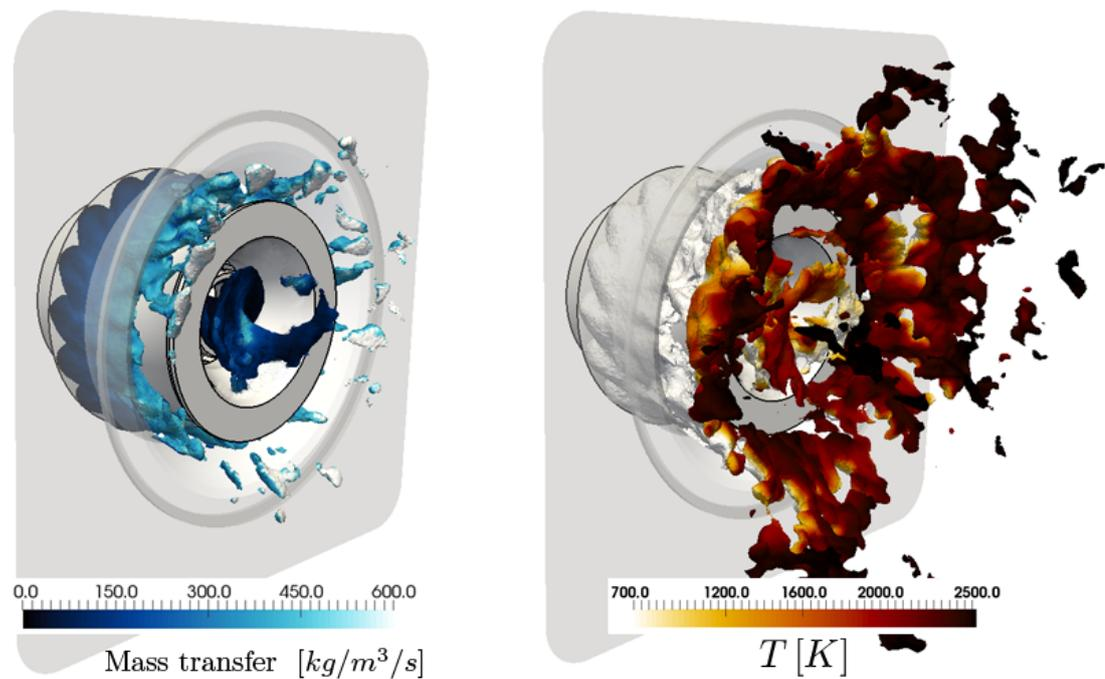
**Figure 10.14:** LEMCOTEC: Left) isosurface of stoichiometric liquid volume fraction coloured by evaporation source term. Right) isosurface of stoichiometric total (liquid + vapor) equivalence ratio coloured by temperature.
