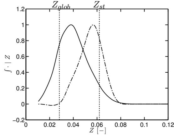
**Figure 10.21: LEMCOTEC: Integrated fuel consumption (—) and NO production (· - ·) conditioned on the mixture fraction vs mixture fraction. The distributions are normalised by their respective peak value. The vertical lines correspond to the global mixture fraction and the stoichiometric mixture fraction.**
