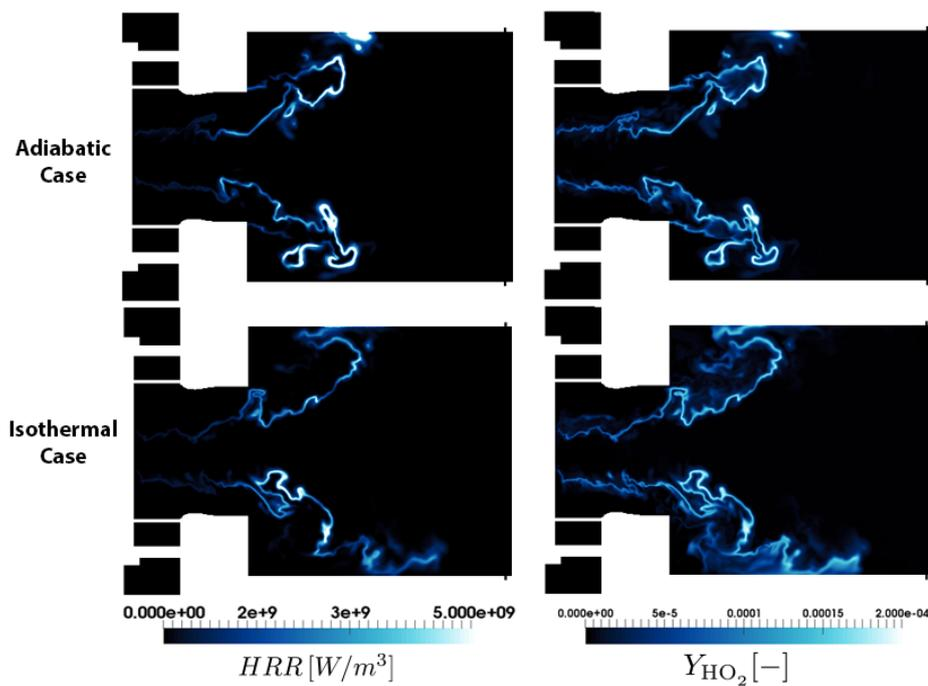
Figure 9.50: SGT-100/Case A: instantaneous fields of heat release rate (left) and  $HO_2$  (right) from LES in the mid-plane of the combustor. Comparison between adiabatic case (top) and isothermal case (bottom).
