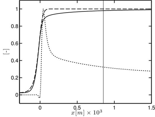
**Figure 5.4: One-dimensional methane-air premixed flame at  $\phi = 1.0$  ( $T = 680$  K and  $P = 3$  bars - SGT-100/Case A conditions). Profiles of progress variable from detailed chemistry (—), two-step GRC  $c_{2s}$  (---) and normalised  $\text{NO}_x$  source term from detailed chemistry ( $\cdots$ ). The vertical line corresponds to the switch value  $c^* = 0.98$ .**
