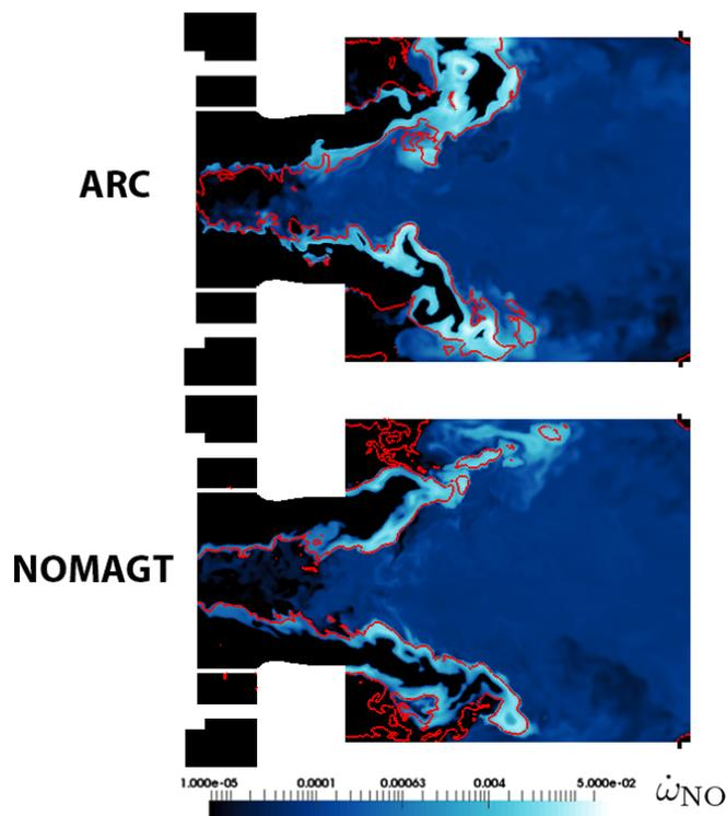
Figure 9.30: SGT-100/Case A - NOMAGT: comparison of instantaneous fields of NO source term ( $\text{kg}/\text{m}^3/\text{s}$ ) between ARC (baseline case) and NOMAGT case in the mid-plane of the combustor. Isocontour of progress variable  $c = 0.98$  for the ARC case, and  $c^* = 0.98$  for the NOMAGT case.
