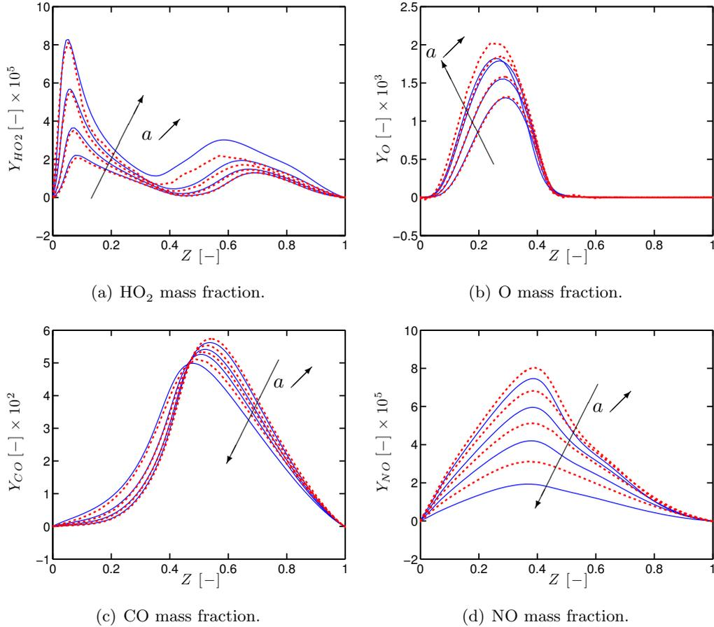
**Figure 7.18: Counterflow computations in Sandia flame D conditions at global strain rates  $a = 40, 80, 160, 320 \text{ s}^{-1}$ . Comparison of species mass fractions from Cantera (—) and AVBP (···) in  $Z$ -space.**
