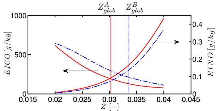
Figure 9.40: CO and NO flame emission indices from unstrained premixed laminar flames vs mixture fraction. Comparison between **Case A** (—) and **Case B** (· - · -). The vertical lines correspond to the respective global mixture fraction of both cases.
