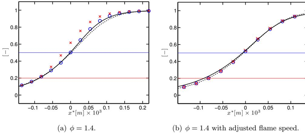
**Figure 5.10:** Comparison of the NOMAGT model with detailed chemistry on a one-dimensional methane-air premixed flame. Impact of  $c_{relax}$  on the progress variable  $c^*$ :  $c_{relax} = 0.5$  ( $\circ$ ), and  $c_{relax} = 0.2$  ( $\times$ ). The progress variable of the reduced chemistry  $c_{2s}$  ( $\cdots$ ) and the detailed chemistry ( $—$ ) are shown for comparison. The switch thresholds are indicated by the horizontal lines.
