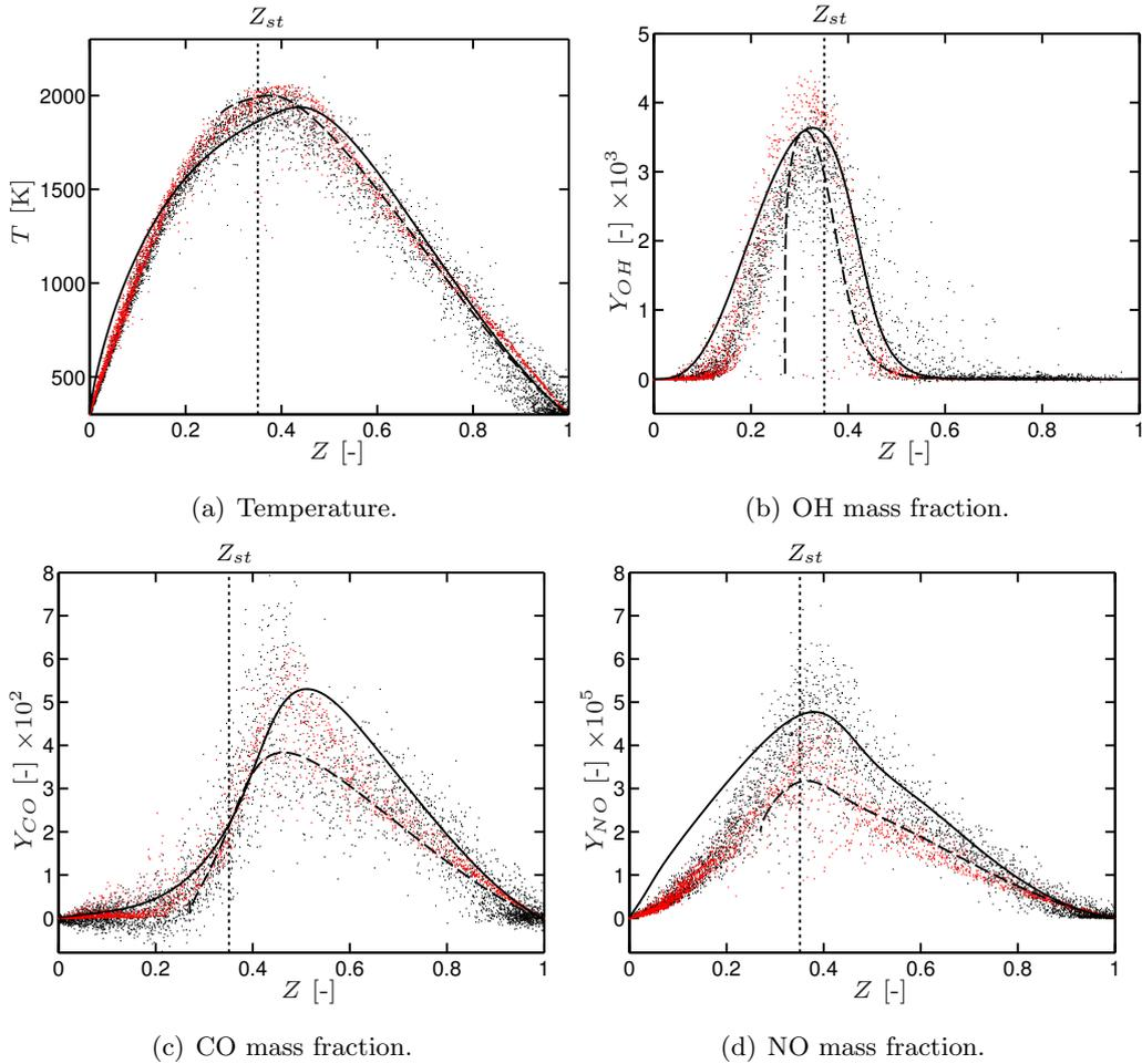
**Figure 8.15: Sandia flame D: Temperature, OH, CO and NO mass fractions vs mixture fraction at axial location  $z = 7.5D$ . Black dot: experiments, Red dot: LES. Coflow counterflow flame (—) and pilot counterflow flame (---) at strain rate  $a = 170\text{s}^{-1}$ .**
