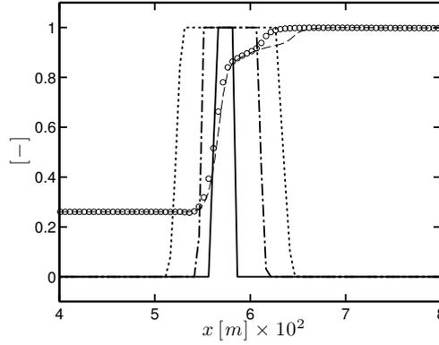
**Figure 6.10:** One-dimensional unstrained premixed laminar flame in SGT-100 Case A conditions at  $\phi = 1.0$ . Unfiltered thickening sensor (—), normalised spatial profiles of temperature with baseline parameters (--) and modified  $Sc_\psi$  ( $\circ$ ), filtered thickening sensor with baseline parameters ( $\cdots$ ) and modified  $Sc_\psi$  ( $-\cdot-\cdot$ ).
