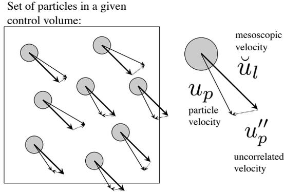
**Figure 3.1:** Decomposition of the particle velocity  $u_p$  into a mesoscopic part  $\check{u}_l$  and an uncorrelated part  $u_p''$ .
