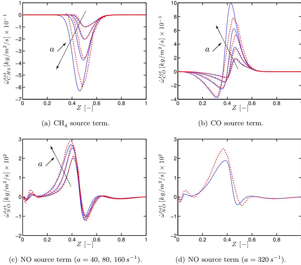
**Figure 7.19: Counterflow computations in Sandia flame D conditions at global strain rates  $a = 40, 80, 160, 320 \text{ s}^{-1}$ . Comparison of source terms from Cantera (—) and AVBP (⋯⋯) in  $Z$ -space.**
