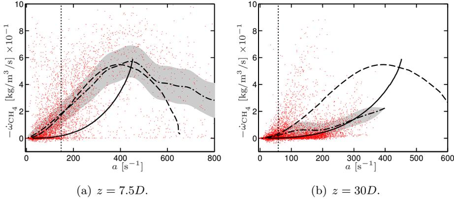
**Figure 8.19: Sandia flame D: Scatter plot of  $\text{CH}_4$  consumption rate versus strain rate along the  $Z = 0.4$  isosurface at axial locations a)  $z = 7.5D$  and b)  $z = 30D$ . The grey shaded area corresponds to the conditional standard deviation around the conditional mean ( $\cdot - \cdot -$ ). The vertical line corresponds to the mean strain rate. LES results are compared to the coflow counterflow flamelets ( $-$ ) and the pilot counterflow flamelets ( $--$ ).**
