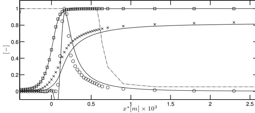
**Figure 5.8:** Comparison of the NOMAGT model with detailed chemistry on a one-dimensional methane-air premixed flame at  $\phi = 1.4$ : normalised profiles of thickening factor ( $-\cdot-$ ), progress variable  $c^*$  ( $\square$ ), NO mass fraction from NOMAGT ( $\times$ ) and NO source term from NOMAGT ( $\circ$ ). The continuous lines corresponds to the results obtained for the detailed mechanism with Cantera.
