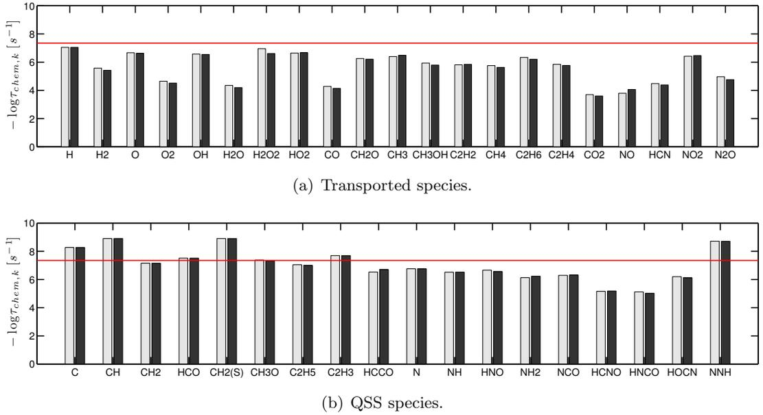
**Figure 7.20: Species chemical times extracted from counterflow flame computations in Sandia flame D conditions at global strain  $a = 40 \text{ s}^{-1}$  (white) and  $a = 320 \text{ s}^{-1}$  (black). The continuous line corresponds to the time-step of the computations ( $\Delta t = 4.5 \times 10^{-8} \text{ s}$ )**
