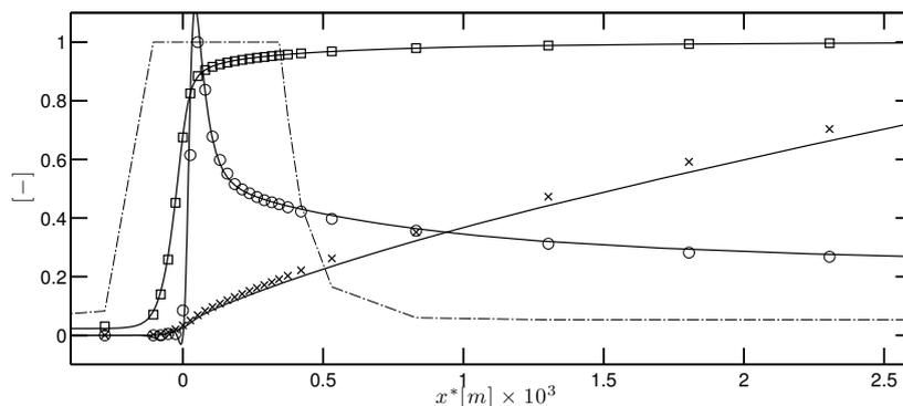
Figure 5.6: Comparison of the NOMAGT model with detailed chemistry on a one-dimensional methane-air premixed flame at  $\phi = 1.0$ : normalised profiles of thickening factor (— · —), progress variable  $c^*$  ( $\square$ ), NO mass fraction from NOMAGT ( $\times$ ) and NO source term from NOMAGT ( $\circ$ ). The continuous lines corresponds to the results obtained for the detailed mechanism with Cantera.
