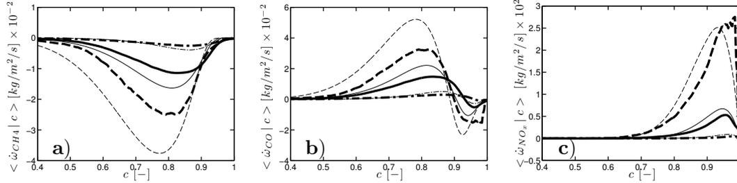
**Figure 9.13: SGT-100/Case A: a)  $\text{CH}_4$ , b)  $\text{CO}$  and c)  $\text{NO}_x$  source terms conditionally averaged on progress variable and on mixture fractions  $Z = 0.025$  ( $\dashv$ ),  $Z = Z_{\text{glob}}$  ( $\rule{0.5cm}{0.4pt}$ ) and  $Z = 0.035$  ( $\rule{0.5cm}{1.2pt}$ ) (bold lines) vs progress variable. Thin lines correspond to the unstrained premixed laminar flame at the same mixture fraction values.**
