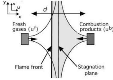
**Figure 4.3: Schematic of a canonical counterflow strained premixed flame.**
