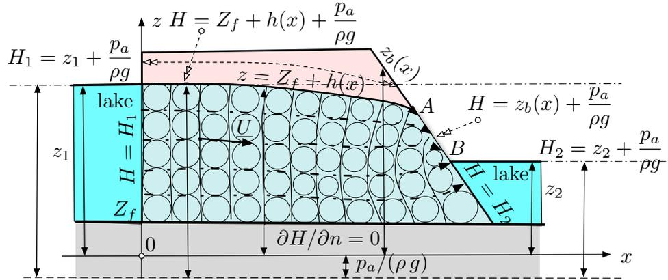
Figure 2.8: Iso- $H$  (solid lines) and trajectories (dot-dashed lines) of in a phreatic aquifer between two lakes.
