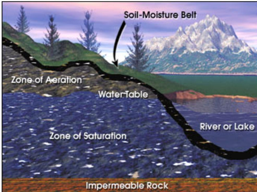
Figure 2.1: *Water table in contact with a river or a lake [NASA GSFC, by Hailey King].*
