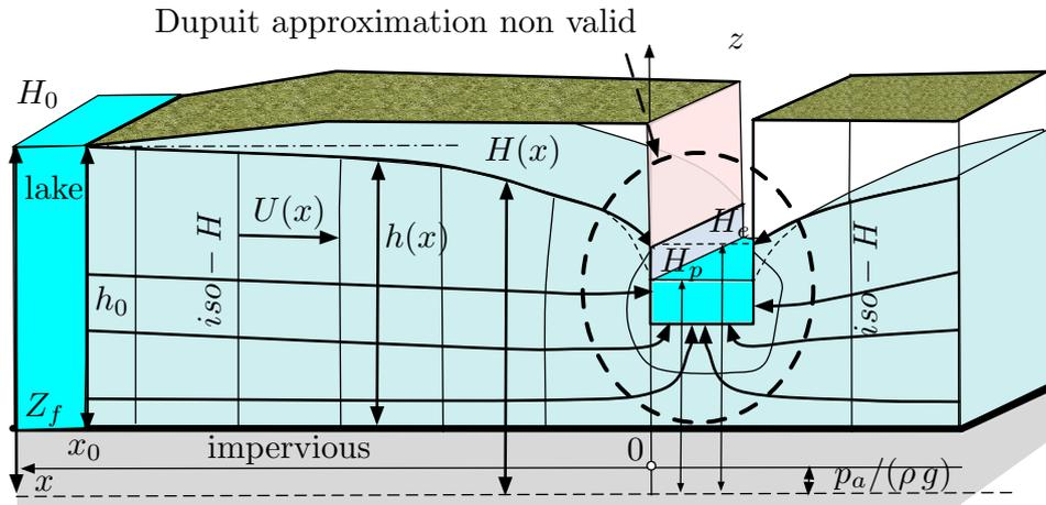
Figure 2.11: Flow towards a **prismatic ditch** in a phreatic aquifer.
