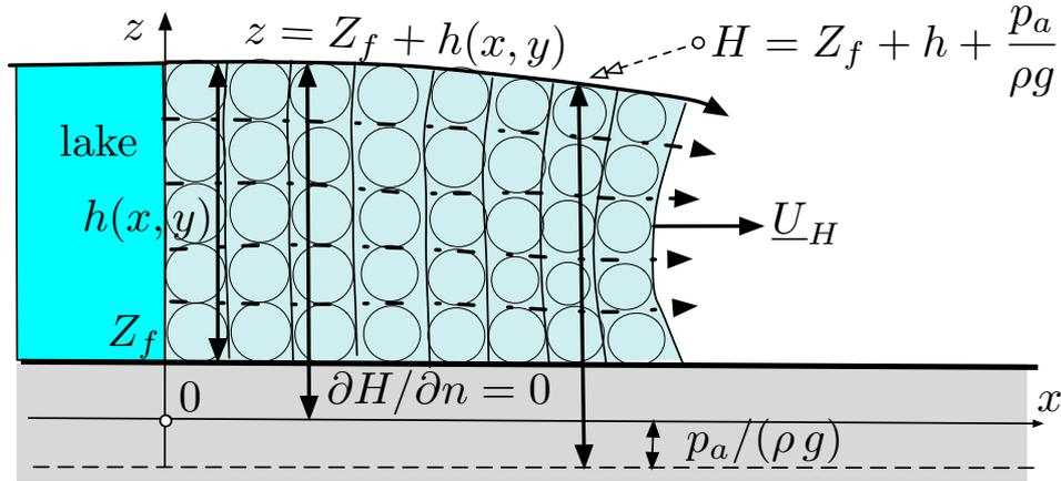
Figure 2.10: Dupuit approximation valid for nearly vertical iso- $H$ .
