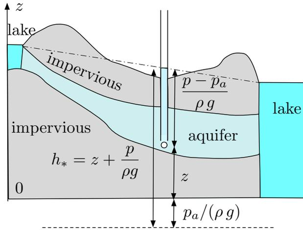
Figure 2.4: Piezometric height  $h_* = \frac{p}{\rho g} + z$  in an aquifer.
