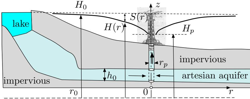
Figure 2.9: *Depression curve  $S(r)$  for an artesian well.*
