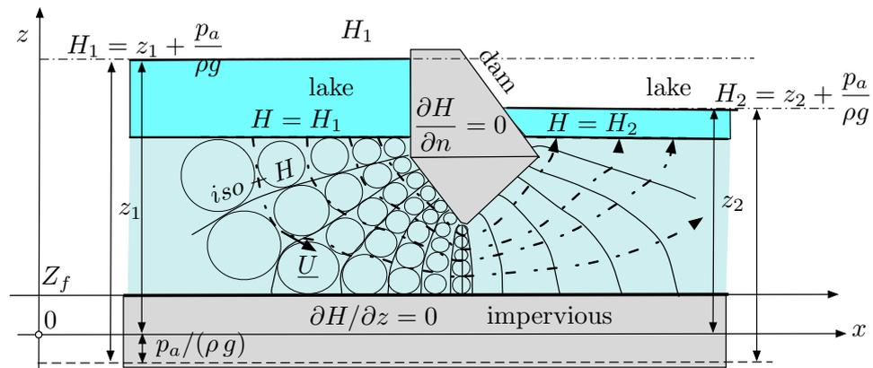
Figure 2.7: *Iso- $H$  (solid lines) and trajectories (dot-dashed lines) of a groundwater flow under a dam.*
