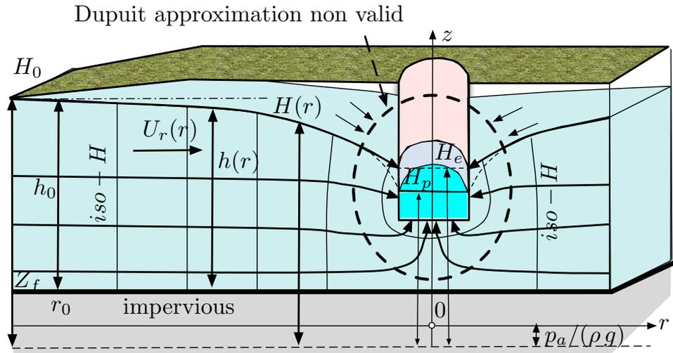
Figure 2.12: Velocity  $\underline{U} = U_r \underline{e}_r$  of a phreatic aquifer around **vertical and cylindrical well**.
