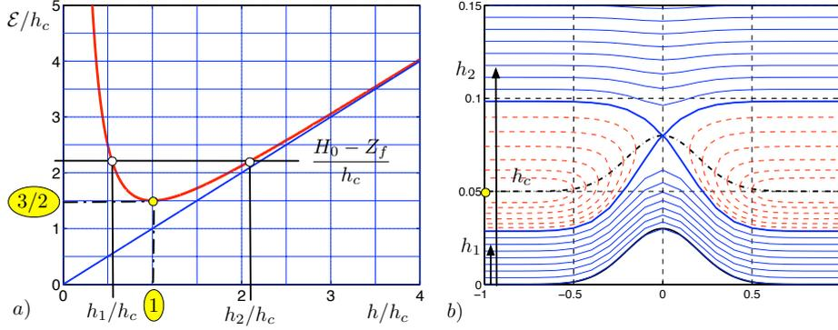
Figure 4.6: a) Dimensionless specific head  $\frac{\mathcal{E}(q,h)}{h_c} = \frac{h}{h_c} + \frac{1}{2} \left(\frac{h}{h_c}\right)^{-2}$  with  $h_c = q^{2/3} g^{-1/3}$ . b) Possible free surface profiles.
