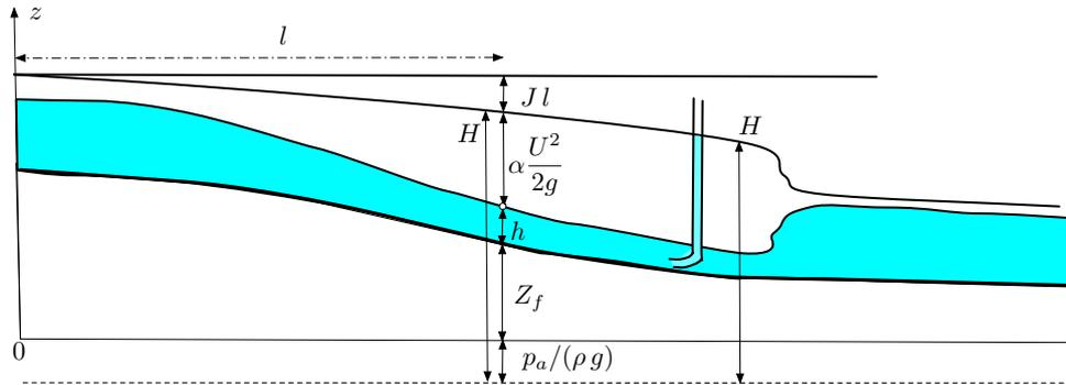
Figure 4.4: Averaged head  $H = \frac{p_a}{\rho g} + Z_f + h + \alpha \frac{U^2}{2g}$  and lineic head loss  $J$ .
