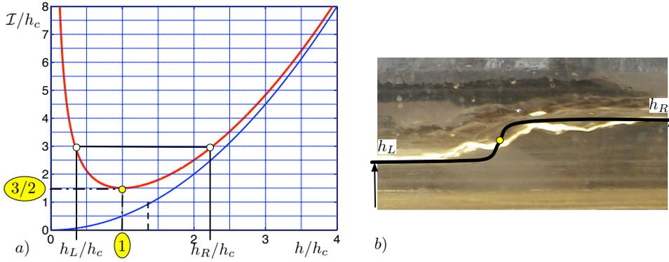
Figure 4.8: a) Dimensionless impulse function  $\frac{\mathcal{I}(q,h)}{h_c} = \left(\frac{h}{h_c}\right)^{-1} + \frac{1}{2} \left(\frac{h}{h_c}\right)^2$  with  $h_c = q^{2/3} g^{-1/3}$ . b) Hydraulic jump.
