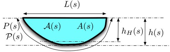
Figure 4.3: Section  $\mathcal{A}(s)$ , wet perimeter  $P(s)$ , top width  $L(s)$ , maximal depth  $h(s)$  and hydraulic depth  $h_H(s)$ .
