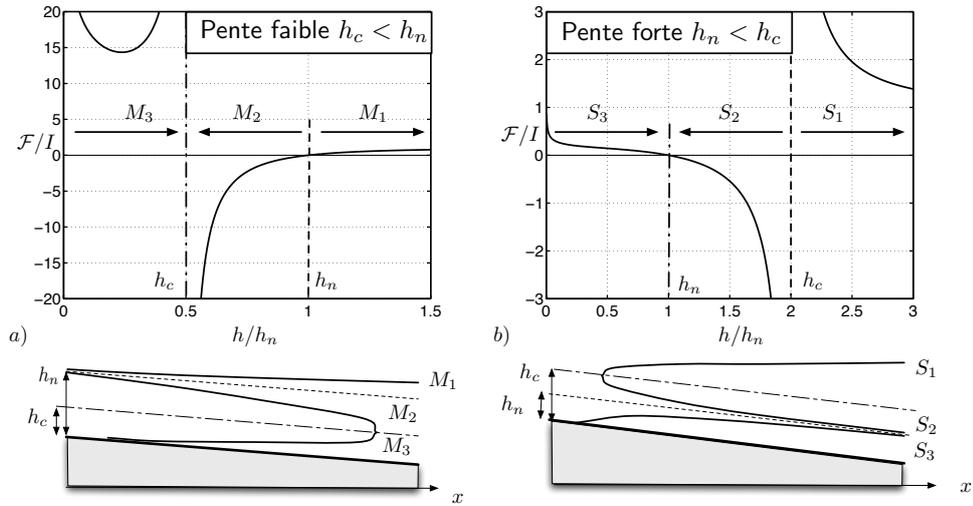
Figure 4.10: Function  $\mathcal{F}(h)$  and associated back water curves  $h(s)$ . a) Weak slope regime  $h_c < h_n$  with type M curves. b) Strong slope regime  $h_n < h_c$  with S curves.
