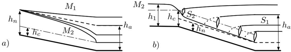
Figure 4.11: Slope changes and associated backwater curves. a) Weak slope regime. b) Strong slope example with hydraulic jump.
