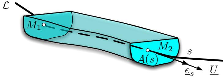
Figure 4.2: Streamline  $\mathcal{L}$  in an open channel flow.
