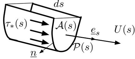
Figure 4.9: Shear stress  $\tau_*$  applied by the flow on the walls of the wet perimeter  $P$ .
