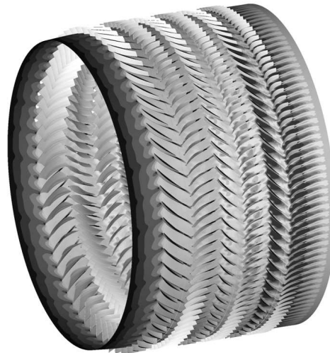
FIG. 3.9 – Whole simulation of the three stages compressor, Instantaneous Axial Velocity Flow Field (black : low velocity, white : high velocity).
