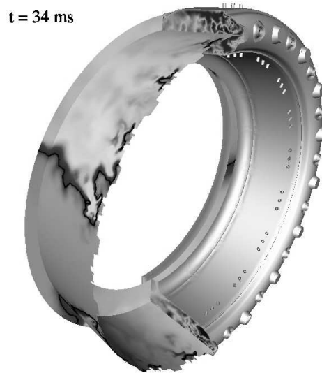
FIG. 3.1 – Temperature field in the combustor at one instant of the ignition sequence (grey : cold - white : hot). The black line is the iso-level T=1500 K locating the flame front which propagates in the azimuthal direction close to the injectors outlets.
