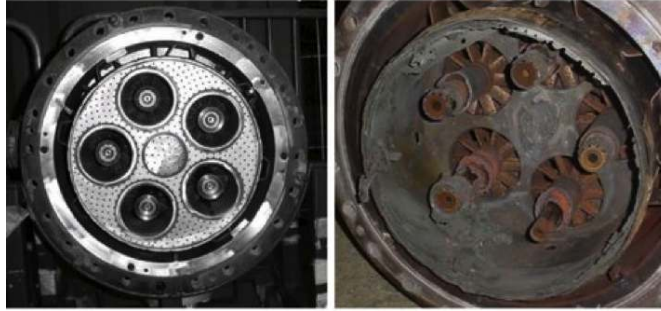
Figure 1.4: A five-burner combustion chamber before (left) and after (right) combustion instabilities.
