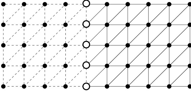
Figure 2.1: Partition of the domain based on an element splitting. Shared vertices are indicated by a circle.
