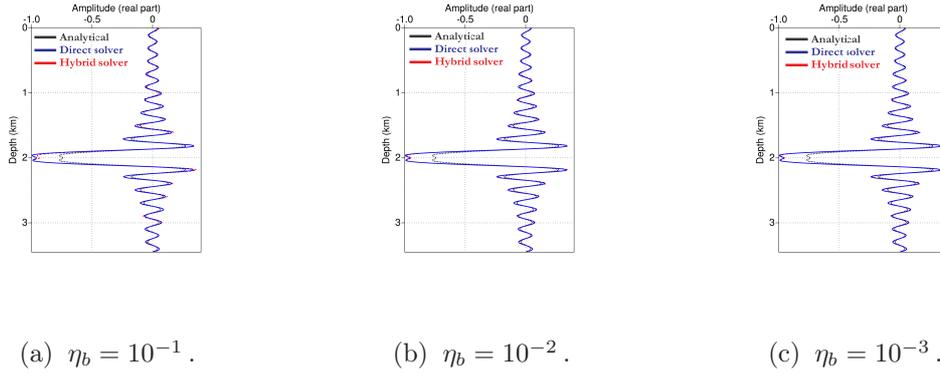
Figure 8.3: Comparison of the solution of a 3D Green function in a homogeneous media for different values of the stopping criterion  $\eta_b$ . Note that a value of  $\eta_b = 10^{-3}$  provides a meaningful solution compared to both the analytical and the direct solutions.
