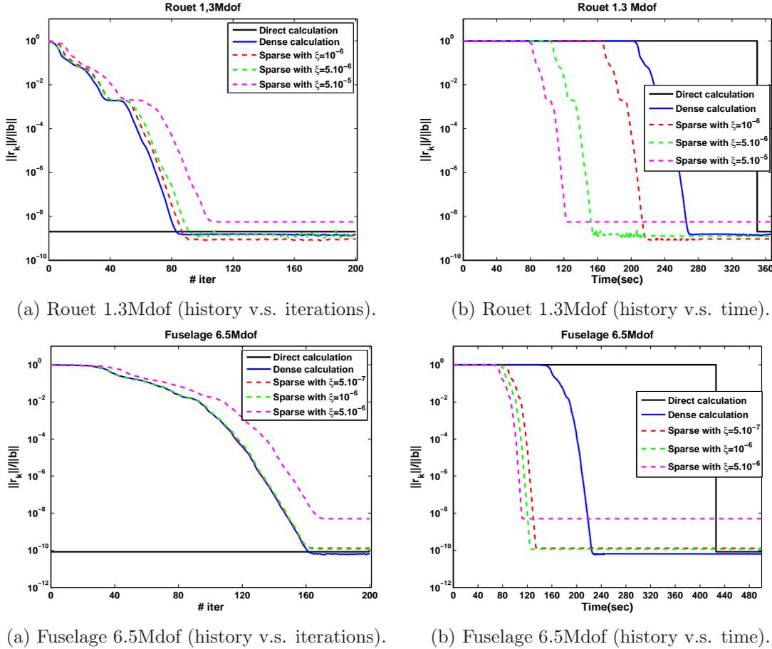
Figure 7.2: Convergence history of full-GMRES for Fuselage and Rouet problems mapped onto 16 processors, of the direct, the Hybrid-dense ( $M_{d-64}$ ) and the Hybrid-sparse ( $M_{sp-64}$ ) solvers for various sparsification dropping thresholds (Left: scaled residual versus iterations, Right: scaled residual versus time).
