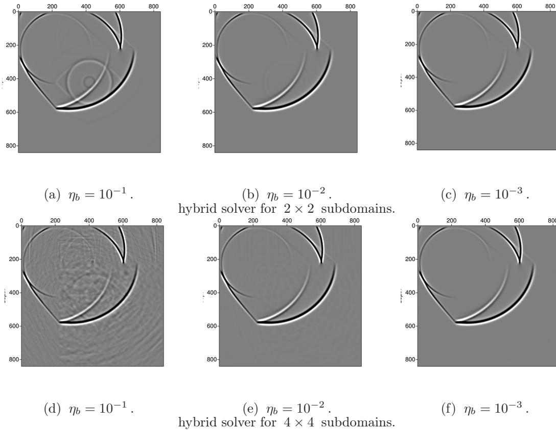
Figure 8.4: Snapshots computed in the corner-edge model with different values of the stopping criterion  $\eta_b$ . Note the diffraction at the intersection between the subdomains for  $\eta_b = 10^{-1}$ .
