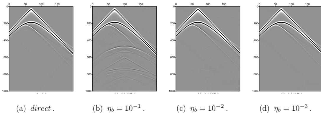
Figure 8.5: Seismograms computed in the corner-edge model with direct solver (a) and with different value of  $\eta_b$  for the hybrid solver.  $\eta_b$  is  $10^{-1}$  (b),  $10^{-2}$  (c) and  $10^{-3}$  (d).
