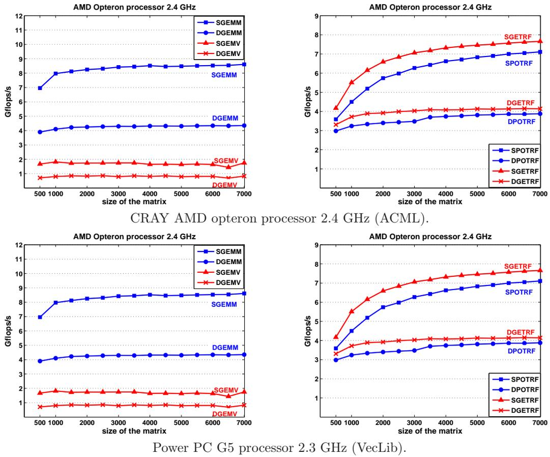
Figure 3.3: Performance comparison of various BLAS-LAPACK Kernels.
