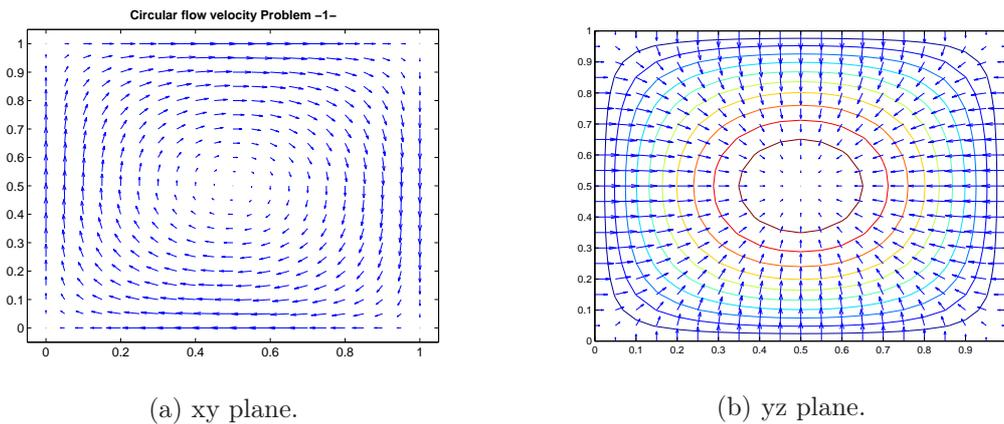
Figure 6.2: circular convection flow.
