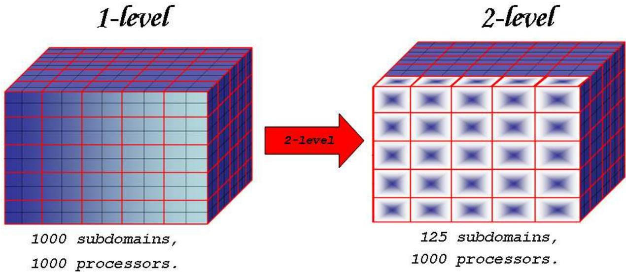
Figure 4.1: Comparison between *1-level parallel* and *2-level parallel* method on 1000 processors, when instead of having 1000 subdomains, we decrease the number of subdomains to 125 while running each one onto 4 processors.
