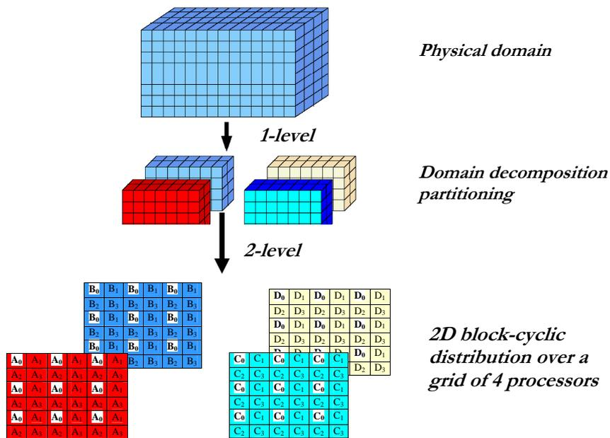
Figure 4.5: Multi-level of data and task distribution.
