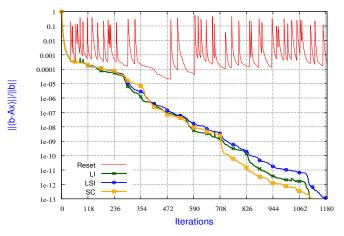
Right block diagonal Preconditioned GMRES on UF Averous/epb0 using 16 cores with 44 faults
