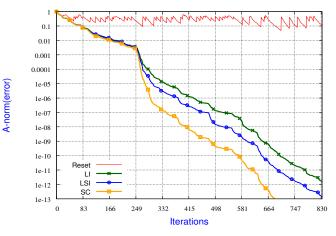
PCG on a 7-point stencil 3D Poisson equation using 16 cores with 70 faults
