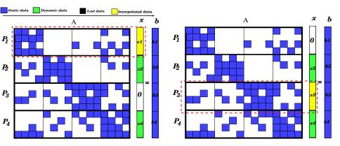
Interpolate  $x_3$  assuming that  $x_1$  is equal to zero subvector. Interpolate  $x_1$  assuming that  $x_3$  is equal to zero subvector.
