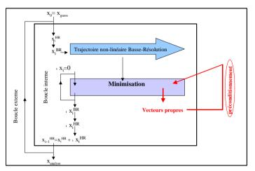
The number of eigen vectors given by the first minimization is roughly equal to (**number of iterations /2**).
