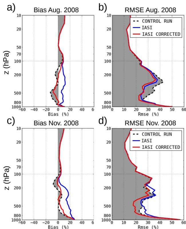
**Fig. 5.** Validation of control run and IASI analyses versus ozonesondes. Same plots as in Fig. 1 (August and November 2008 from top to bottom). Red curves are obtained removing 10 % of the IASI ozone values before the assimilation.
