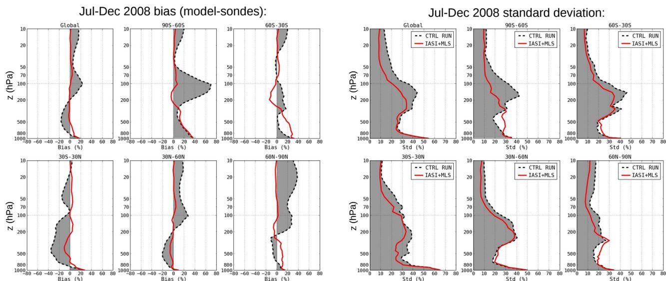
**Fig. 13.** Global and zonal validation of MLS+IASI analysis versus ozonesonde profiles for the long analysis run (July–December 2008). Leftmost 6 panels: bias (model minus sondes) normalized with the climatology (control run in black, analysis in red). Rightmost 6 panels: standard deviation normalized with the climatology.
