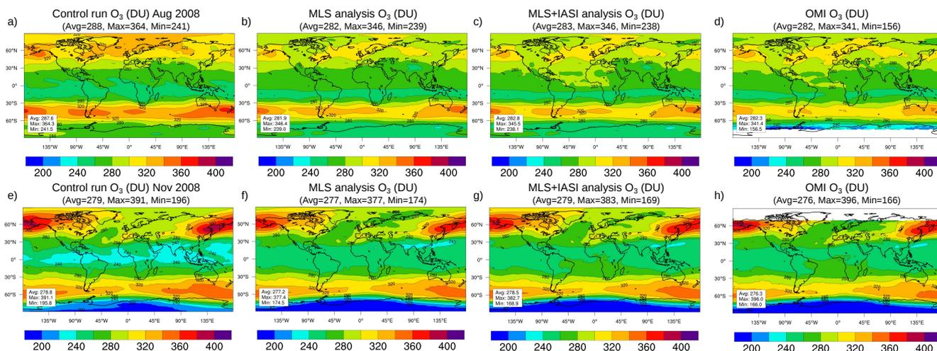
**Fig. 9.** Validation of model total ozone columns versus OMI measurements: (a) control run average ozone column for August 2008, (b) MLS analysis for August 2008, (c) MLS+IASI analysis for August 2008, (d) OMI measurements for August 2008, (e, f, g, h) the same plots but for November 2008. Blue/purple color is reserved for values lower/greater than 200/400 DU. White color in (d, h) indicates pixels without OMI observations.
