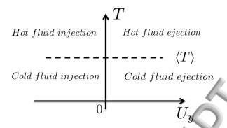
FIG. 16: Representation of the 4 quadrants in the  $(U_y, T)$  space. Injection and ejection events are identified respectively by  $U_y < 0$  and  $U_y > 0$ . Hot and cold events are identified respectively by  $T > \langle T \rangle$  and  $T < \langle T \rangle$ , where  $\langle T \rangle$  is the time and azimuthal averaged local temperature.
