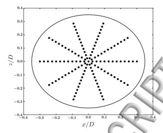
FIG. 13: Location of the numerical probes in the  $(z/D,\,x/D)$  plane used for the PDF analysis. The probes are located at y/D=0.01 for the near wall investigation and at y/D=0 for the analysis of the wall heat flux.
