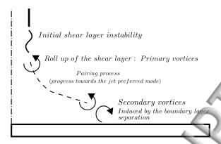
FIG. 9: Description of the large scale structures present in impinging jet flows.
