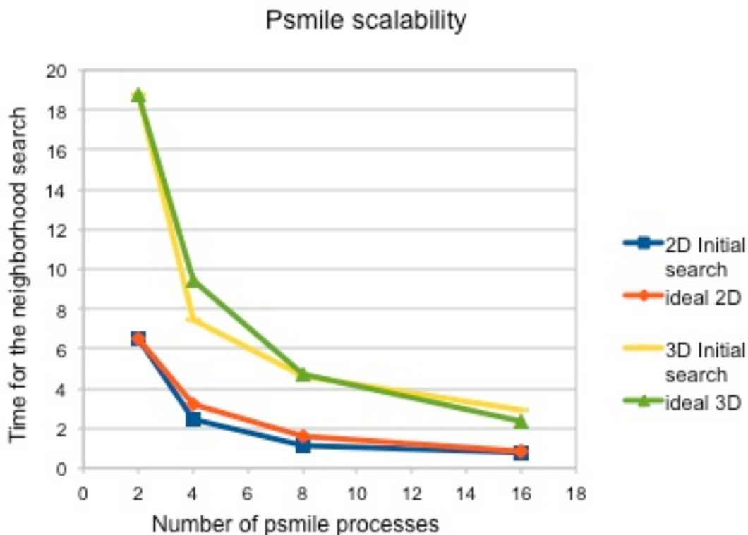
Figure 2 – Time to perform the neighbourhood search as a function of the number of PSMILe processes for the 2D and 3D cases. Ideal curves suppose that the time decreases by a factor X when the number of processes is increased by the same factor X.
