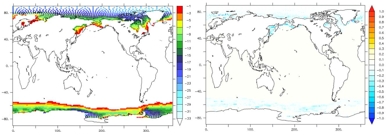
Figure 3: One year average of reconstructed ice temperature (C°) from exchange grid contributions (left) and difference between ice category temperature reconstruction and previous exchange grid result (right). Values calculated on atmosphere grid.
