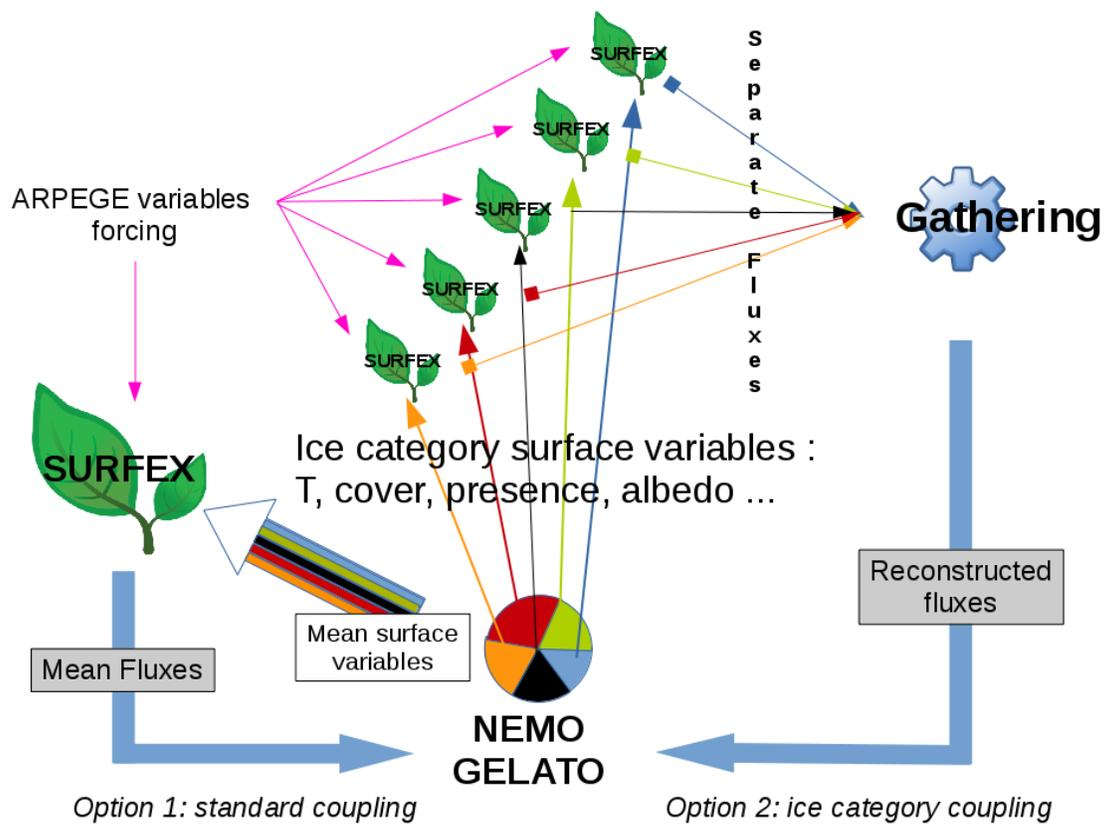
Figure 1: Coupled system implemented to execute n parallel flux calculation with n SURFEX for n ice category surface variables
