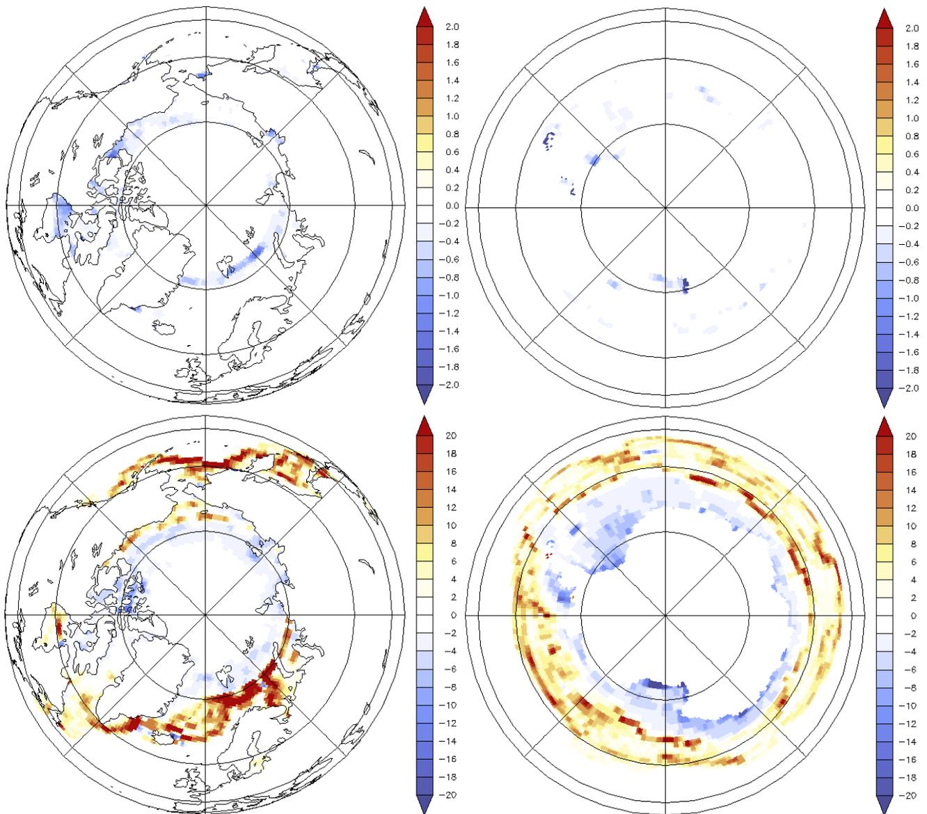
Figure 6: Solar over ice ( $W/m^2$ , upper) and non solar over ice (lower) flux differences (calculated with multi-ice category surface variables - calculated with averaged surface variables) during multi-ice category simulation exchanging multi-ice category surface variables (SMI - STI), annual average, flux interpolated on ocean grid
