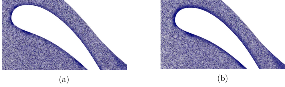
Figure F.1 – View of user-defined mesh (a) and adapted mesh (b) at mid-height of NGV1.
