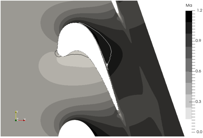
FIGURE 5: Time averaged of Mach number field at mid-span. Isocontour of Ma = 1 is plotted in white. Isocontour of null axial velocity is plotted in black.
