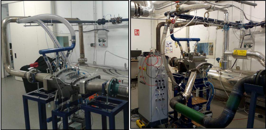
**Figure 1.8:** Trisector test rig at the University of Florence without (left) and with (right) fitted high pressure vane cascade [14].
