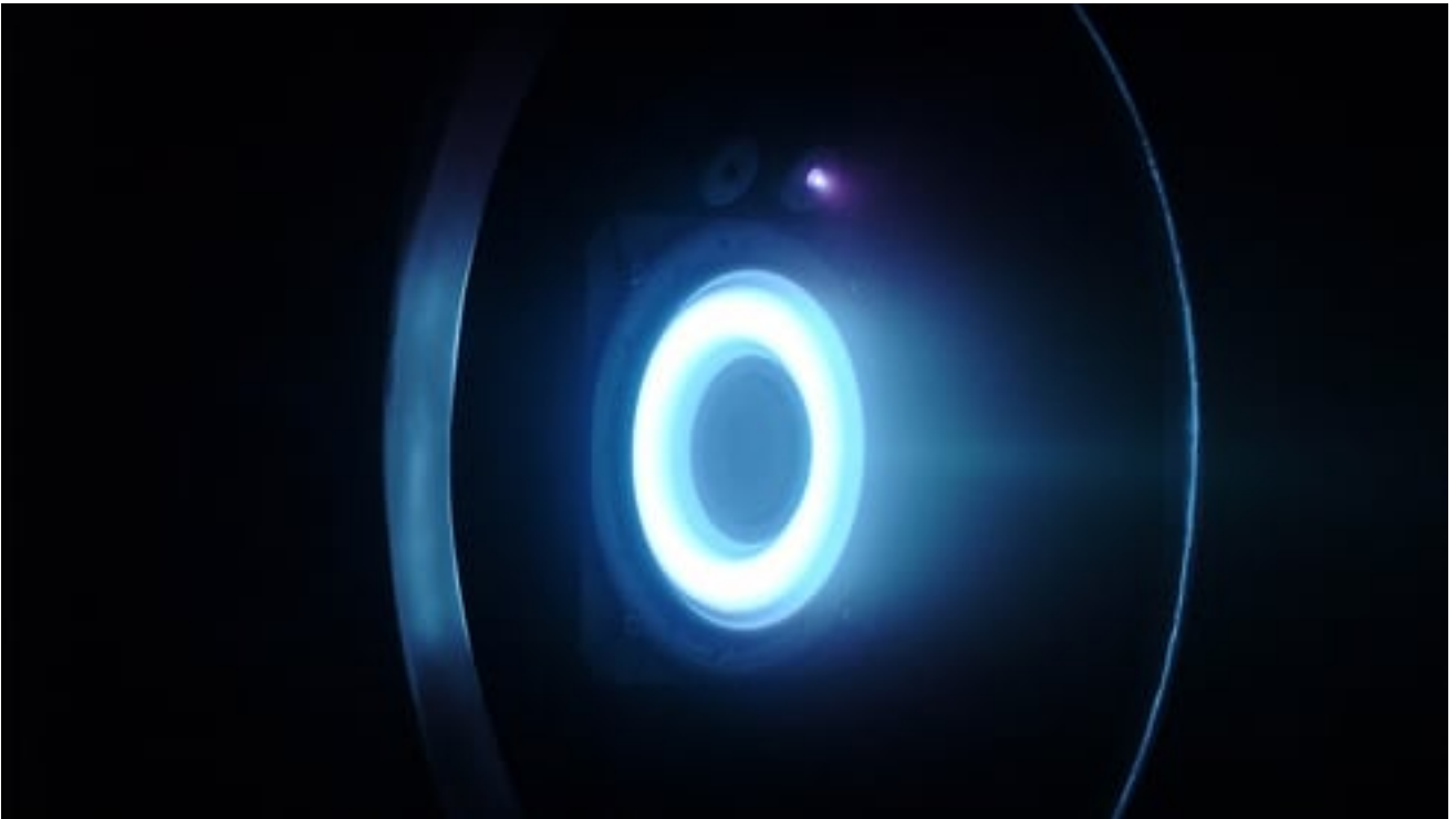
Figure 1.6: PPS-1350 HTs used for the SMART-I mission (Credits Safran Aircraft Engines). The cathode is visible above the thruster.
