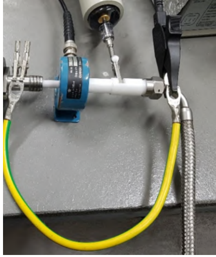
Figure 5: Adaptation to measure temporal current and voltage evolution
