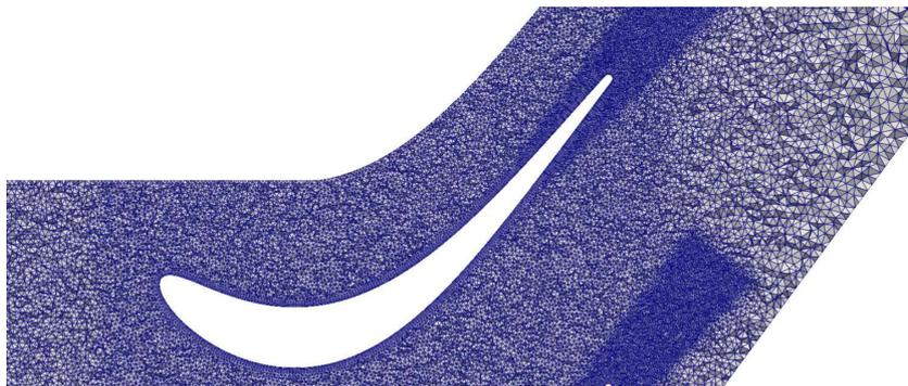
Figure 8: A crinkle-slice focused on one of the blades at  $z/H = 0.5$ , Mesh P, zoomed out.
