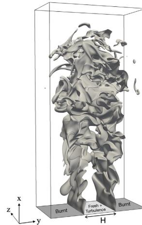
Fig. 1. Physical domain of 3D DNS cases. The inlet contains a central region of width  $H = L_y/3$  with fresh gases at bulk velocity  $U_{bulk}$  and velocity fluctuations  $u'$  (homogeneous isotropic turbulence) surrounded by two laminar coflows at equilibrium state and velocity  $U_{coflow}$ .
