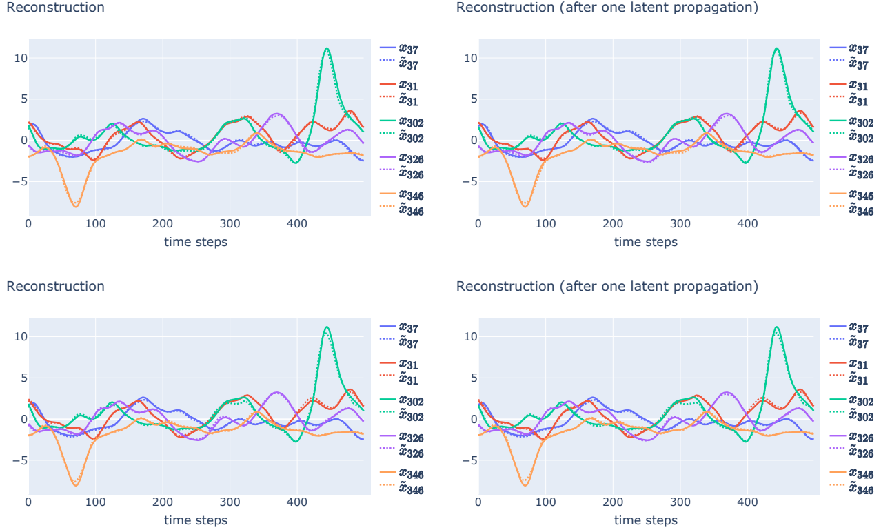
Figure 5.1.29: Top left: reconstruction of five out of 400 variables by the 1-Lipschitz trained network from a simulation in the test dataset, using only the autoencoder. Top right: same as top left plot, but with one latent propagation. Bottom left: reconstruction of five out of 400 variables by the ext-Lipschitz trained network from a simulation in the test dataset, using only the autoencoder. Bottom right: same as bottom left plot, but with one latent propagation. Ground truths are represented by a solid line, and reconstructions with a dashed one.
