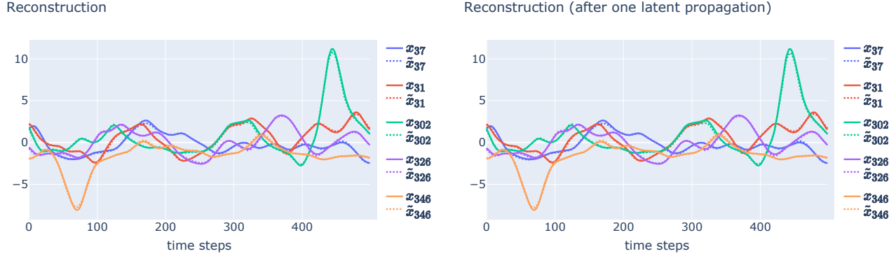
Figure 5.1.16: Left: reconstruction of five out of 400 variables from a simulation in the test dataset (the same one as in Figure 5.1.10) using only the autoencoder, produced by the one-step neural network. Right: the same reconstruction as in the left plot, but with one-step latent propagation also performed. Ground truths are represented by solid lines, and reconstructions by dashed lines.
