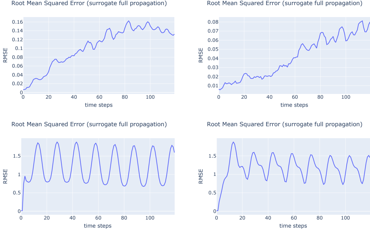
Figure 5.2.20: Top left: RMSE between a ground truth simulation from the training dataset and its full reconstruction by the one-step trained neural network over 120 time steps. Top right: same as top left, but for the experiment involving the two-step surrogate network. Bottom left: same as top left, but for the experiment involving the 1-Lipschitz surrogate network. Bottom right: same as top left, but for the experiment involving the ext-Lipschitz surrogate network.
