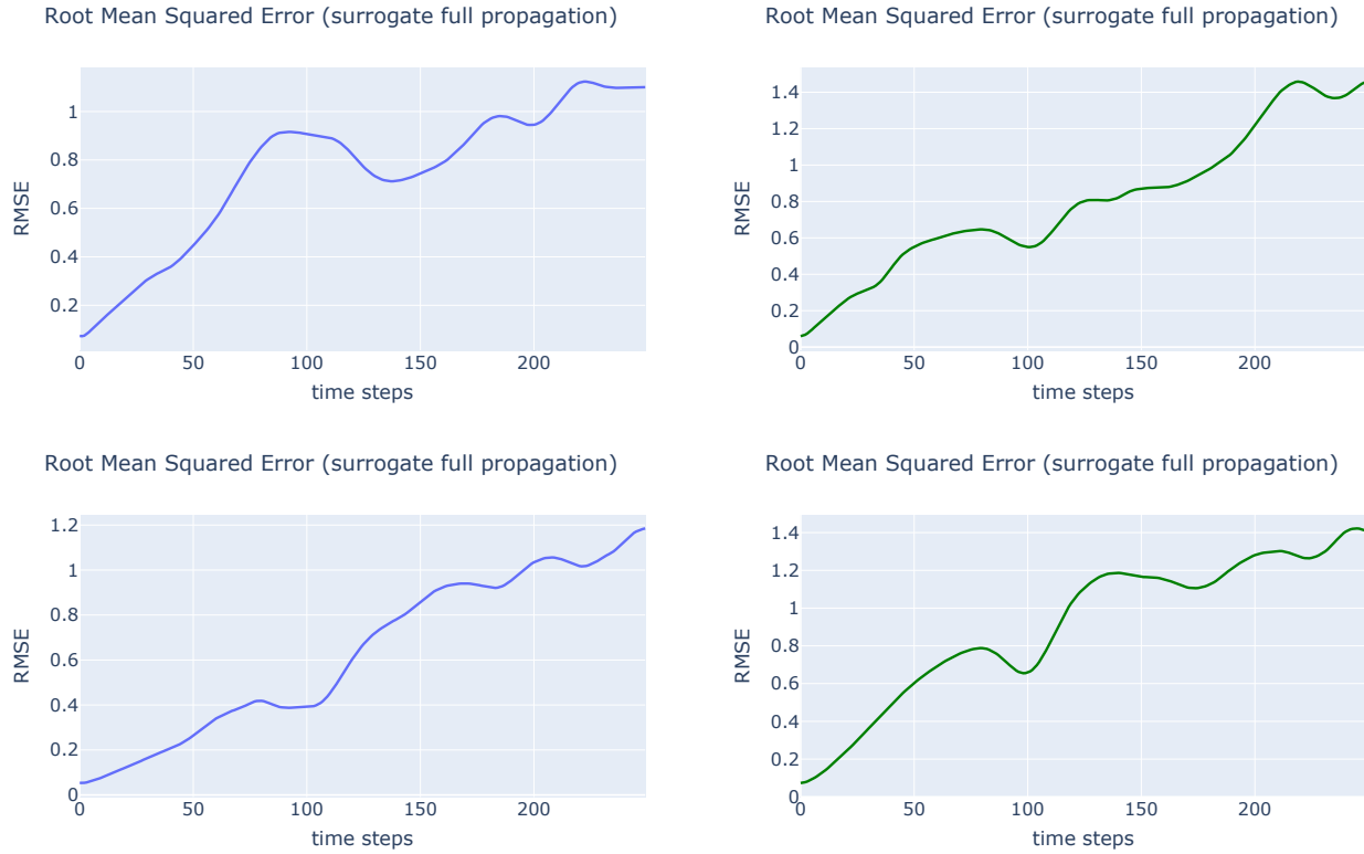
Figure 5.1.23: Top left: RMSE between a ground truth simulation from the training dataset and its full reconstruction by the two-step trained neural network over 250 time steps from \boldsymbol{x}_0 . Top right: RMSE between a ground truth simulation from the test dataset and its full reconstruction by the two-step trained neural network over 250 time steps from \boldsymbol{x}_0 . Bottom left: same as top left but with the initial state set as \boldsymbol{x}_{250} . Bottom right: same as top right, but the initial state set as \boldsymbol{x}_{250} . Blue and green colors are used to differentiate between training (blue) and test (green) data.
