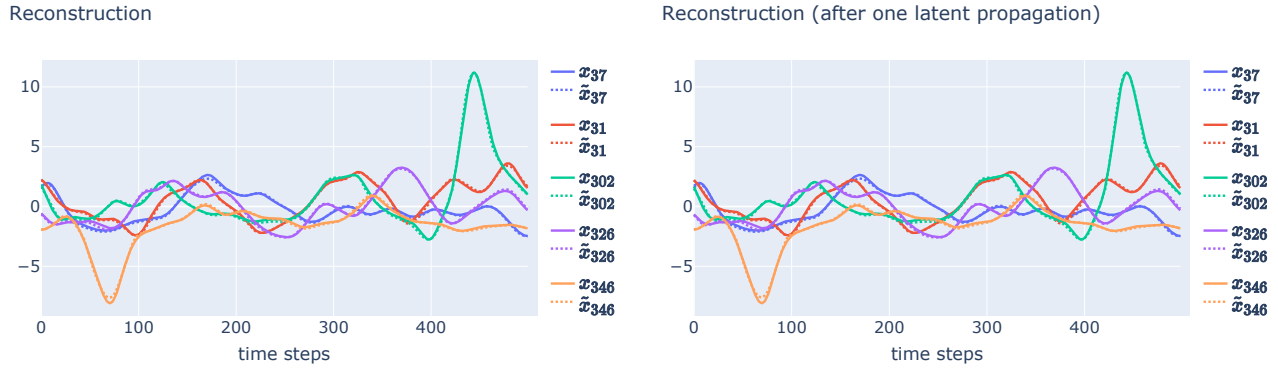
Figure 5.1.11: Left: reconstruction of six out of 400 variables from a simulation in the test dataset (the same one as in Figure 5.1.10) using only the autoencoder. Right: the same reconstruction as in the left plot, but with one-step latent propagation also performed. Ground truths are represented solid lines, and reconstructions with dashed lines.
