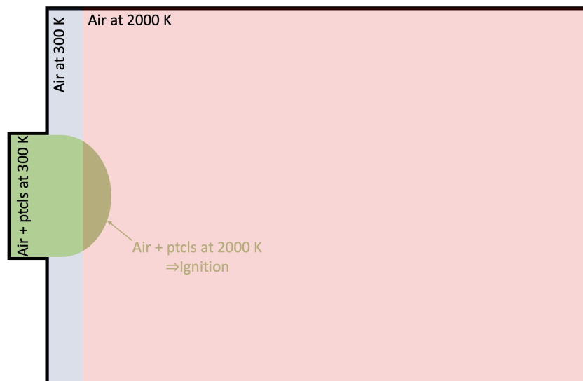
Figure 6.2 – Schematization of the ignition process used in the domain.
