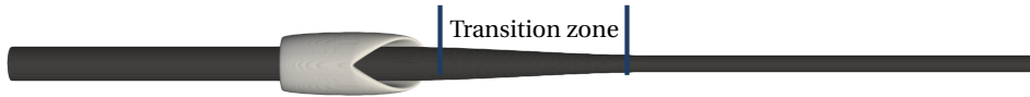
Figure 7.13: Geometry of the inner tube in the simulation domain for a pipe ratio of d^* = 0.25 with the transition region indicated. Note that gravity is applied along the pipe axis so that the case is representative of a vertical pipe configuration.
