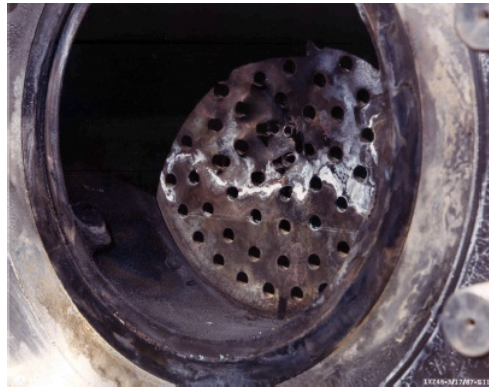
Figure 1.9: Damaged rocket chamber from combustion instabilities.
