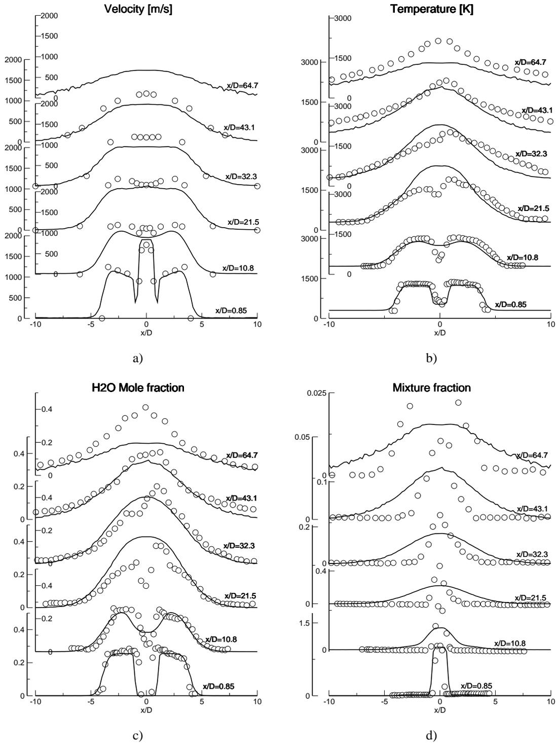
Figure 5: Mean profiles for six transversal planes. Symbols: expt, line: LES.
