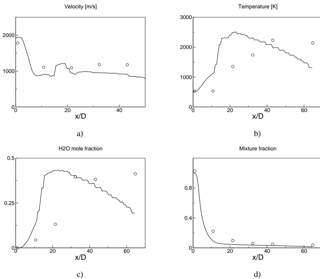
Figure 4: Mean profiles on the longitudinal axis. Symbols: expt, line: LES.
