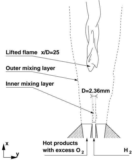
Figure 1: Sketch of Supersonic Burner installed at NASA Langley Research Center
