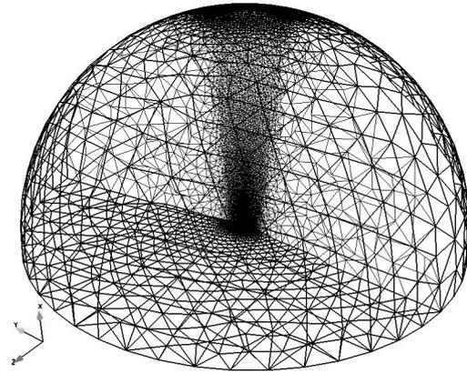
Figure 2: Skin and middle plane of the unstructured mesh
