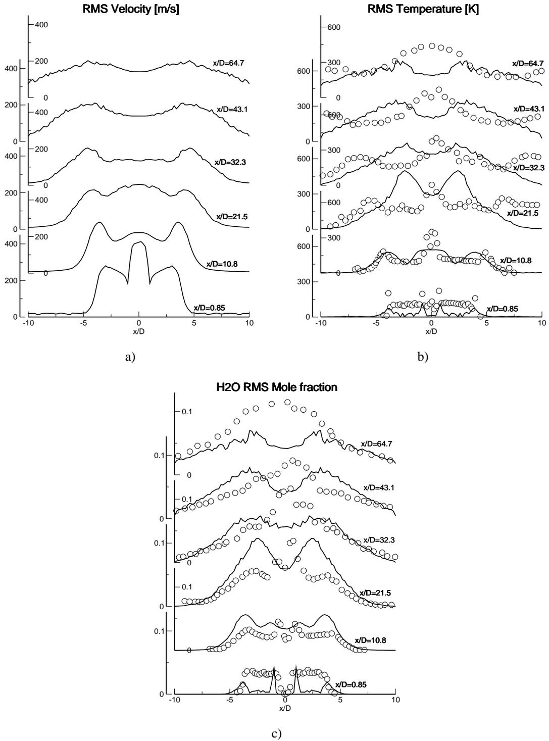
Figure 6: Root Mean Square profiles for six transversal planes. Symbols: expt, line: LES.
