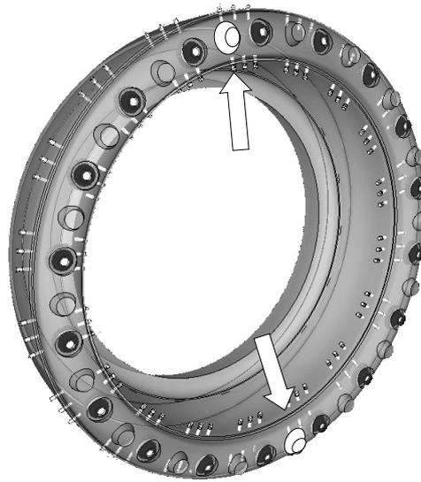
**Fig. 7 Computing domain and boundary conditions of the full combustor (Case F). White arrows point the hot jets location.**
