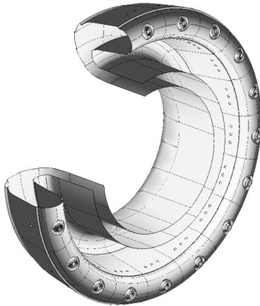
**Fig. 1** Global view of the Vesta combustor (14 of the 18 sectors are represented).
