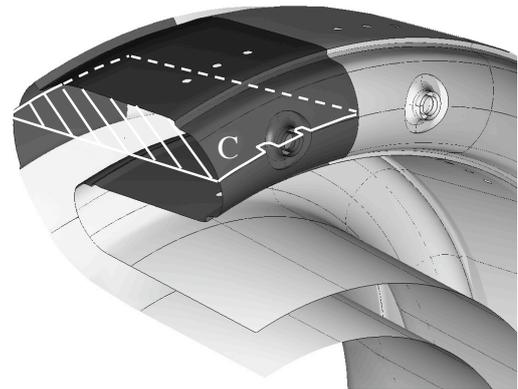
**Fig. 2** Zoom on two sectors: limit of the computational domain (in dark) and cutting surface C (in white).
