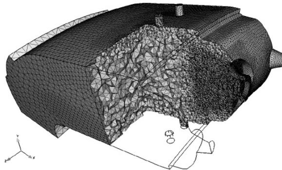
**Fig. 6** View of the computing tetrahedral grid
