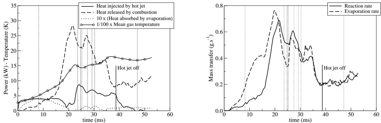
**Fig. 8** Temporal evolution of various total quantities in the domain. Left: energy transfers and gas temperature. Right: mass transfers. The vertical lines indicate the instants of the 9 snapshots featured in Fig. 9.
