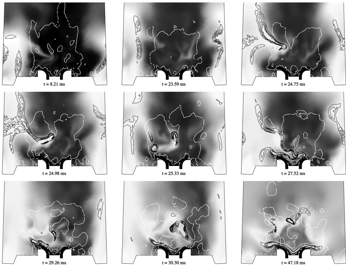
**Fig. 9 Propagation of the reactive zone from the hot jet to the main injector on cutting surface C. Grey scale: gas temperature (black: 273 K → white: 2400 K). Black lines: reaction rate isolines. White lines: back flow lines.**
