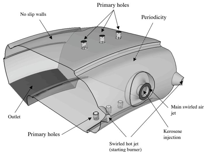
**Fig. 5 Computing domain of the single sector calculation (Case S)**
