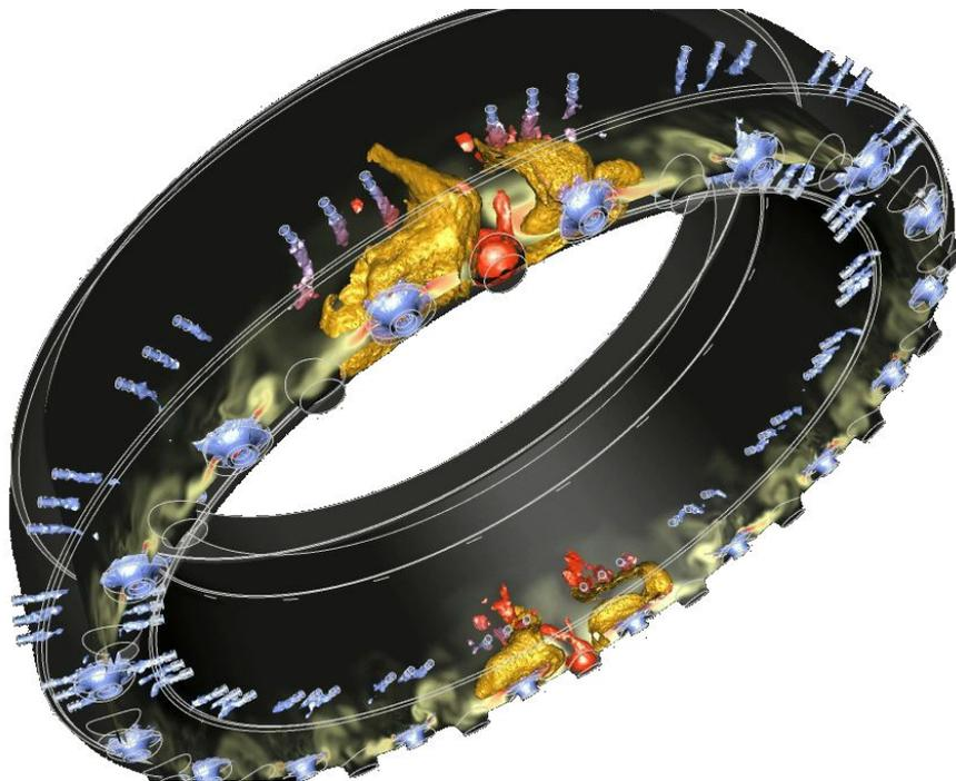
**Fig. 10** Ignition of the full Vesta combustor. Color scale on clipping surface: fuel mass fraction. Bleu surfaces: cold air inlets. Red surfaces: hot jets. Golden surfaces: flame.
