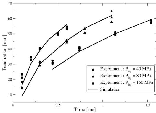
**Figure 1.** Comparison of penetration between simulation and experiment for cases T4P4, T4P8 and T4P15.
