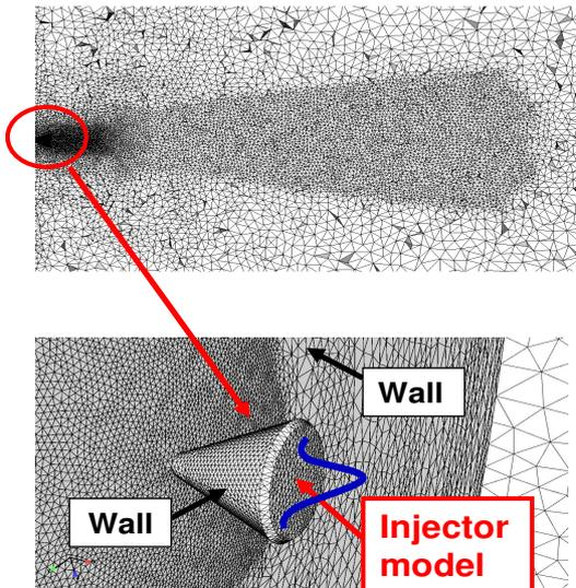
**Figure 5.** Cross section of the mesh and view of the cone dedicated to the shifted boundary condition
