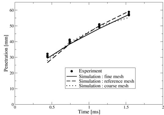
**Figure 4.** Comparison of penetration between simulation and experiment for T4P4 case: Effect of grid resolution.
