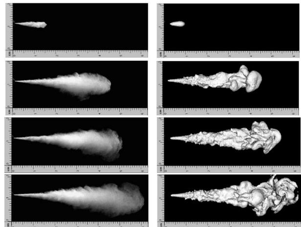
**Figure 6.** Visualization of the spray for the T4P8 case. Comparison between experiment (left) and iso-surfaces of droplet diameter ( $d=3\mu\text{m}$ ) obtained with LES (right) at different times ( $t=0.1\text{ms}$ ,  $0.6\text{ms}$ ,  $0.8\text{ms}$  and  $1.1\text{ms}$ )
