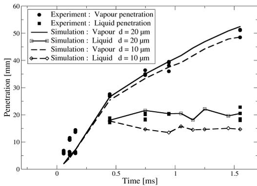
**Figure 3.** Comparison of vapour and liquid penetrations between simulation and experiment for T8P4 case.
