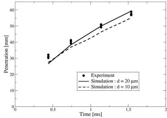
**Figure 2.** Comparison of penetration between simulation and experiment for T4P4 case: Effect of maximum droplet diameter.
