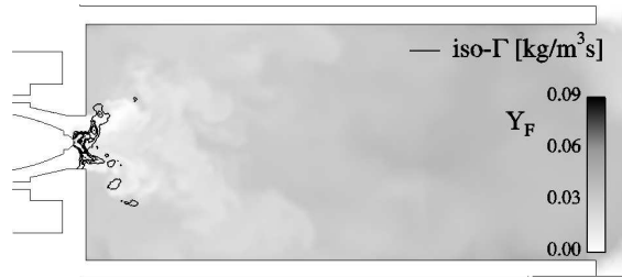
(b) CDP-EL: kerosene vapor and evaporation rate
