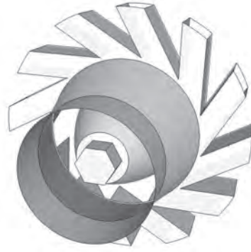
(b) Modified nozzle geometry for the EE approach.
