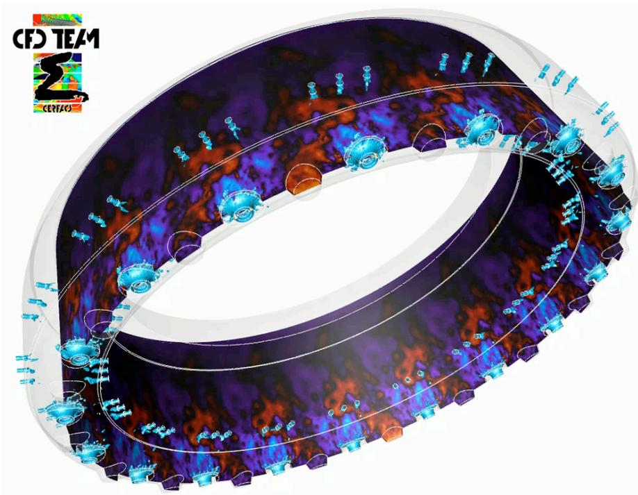
*Thermo-acoustic oscillation in ramjet burner*
