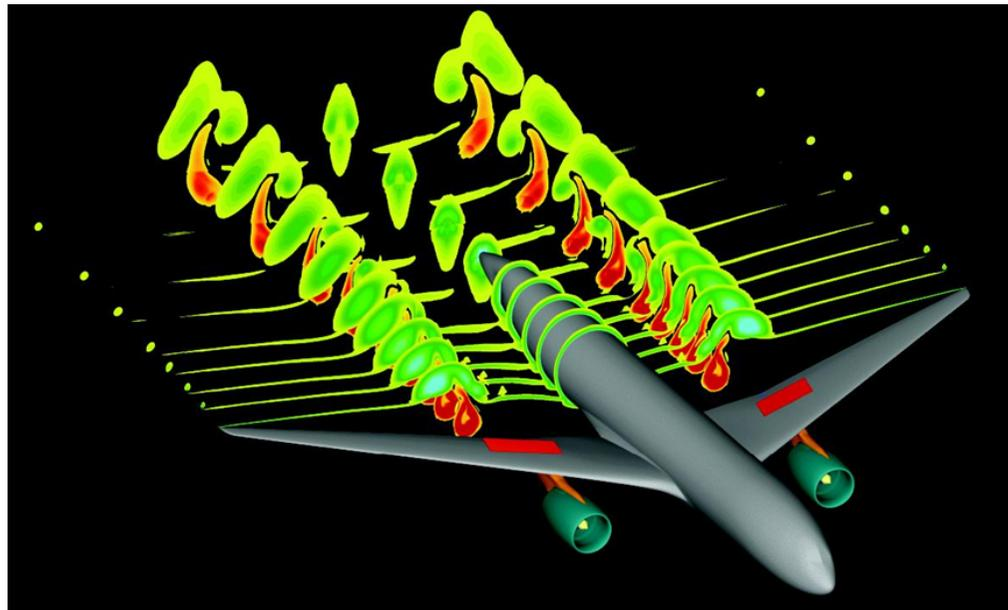
Aeroelastic effects computed with the TSM (including spoilers) in a whole generic long range aircraft performed with e/sA
