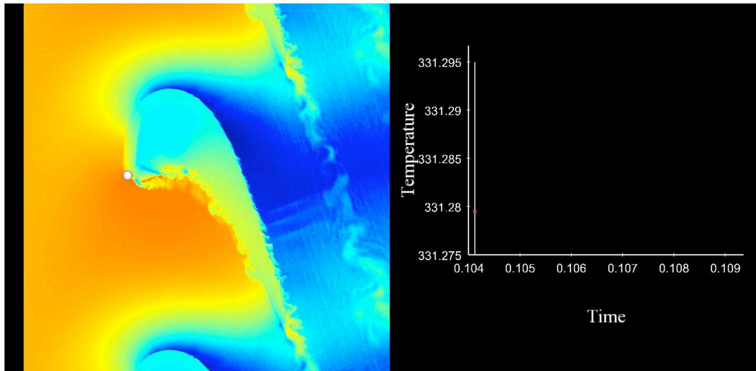
Evolution of flow temperature in the turbine passage
