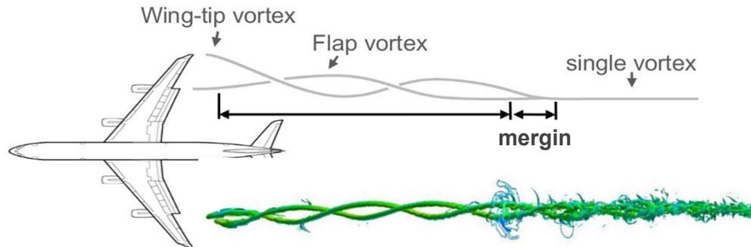
Simulation of wake vortex instabilities behind aircraft (Nybelen et al., 2008):
