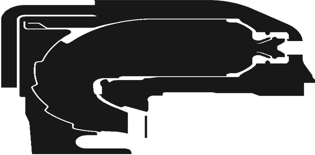
Figure 3. Cut plane of the computational domain for soot prediction in a sector of an annular combustion chamber of a helicopter engine.
