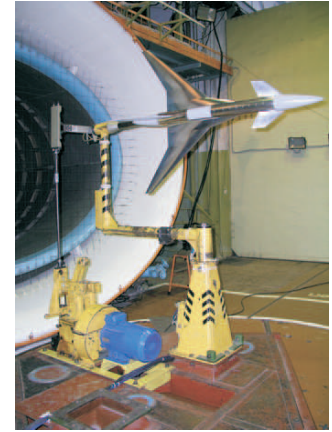
Figure 21. TCR model on the small amplitude roll motion mechanism.
